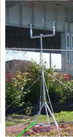
Portable Meteorological Station
