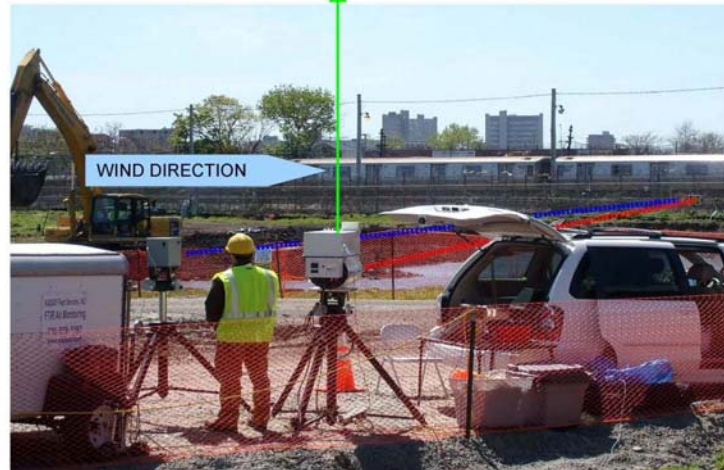
Open-Path FTIR (right) and UV (left) Spectrometers
