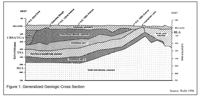
CU1 is estimated to be more than 60 ft thick beneath the southern portion of the site. It gradually thins to less than 15 ft in thickness north of the site, being thinner near the erosional boundary. CU1 is 40 to 45 ft thick near the north property boundary. It consists of interbedded siltstone and claystone; sandstone interbeds are common within CU1.
