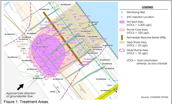
The final plan was to install a permeable reactive barrier downgradient from the source area and perpendicular to the groundwater flow, in order to reduce the contaminant flux that could enter the Mare Island Strait. The source zone, plume core, and near shore area would be treated by injecting EHC<sup>®</sup> into the saturated zone followed by a solution of cheese whey, nutrients and base for pH control (Figure 1).
