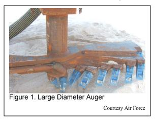
Mixing the ZVI into the soil column solves the contact problem and provides a long term treatment source.
