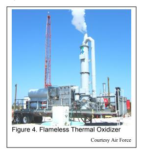
**Project Results:** Approximately 13,272 lbs, 389 lbs, and 11,439 lbs of total VOCs were recovered from SLC-15, SPCC, and Facility 1381, respectively. The cleanup cost averaged at \$190/yd<sup>3</sup>. A remedial efficiency of greater than 99.8% was found for both soil and groundwater. Post treatment sampling one year after remediation showed no rebound or back diffusion. Monitoring wells at Facility 1381 that showed values of up to 800 mg/L of TCE in 2006 before the
