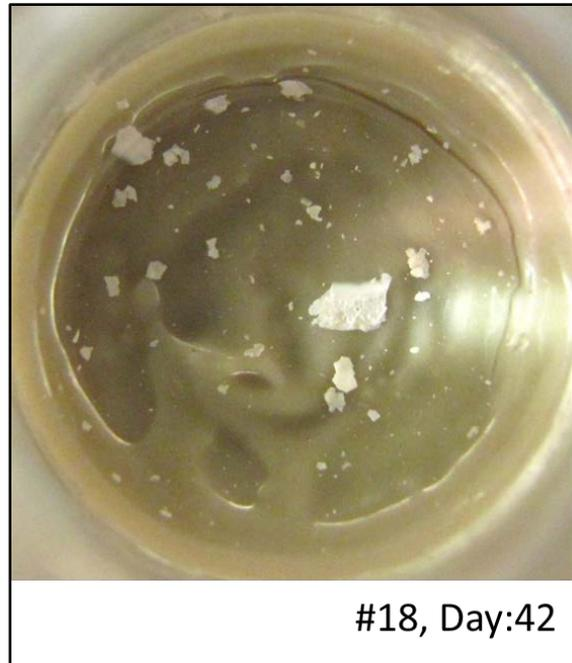
**Figure 4.2.** A mixture of propanol, acetone, methyl isobutyl ketone, 2-butoxyethanol, amyl acetate, and n-butyl acetate dissolved in PCE ponded on water-saturated bentonite for 42 days. No cracking was observed.
