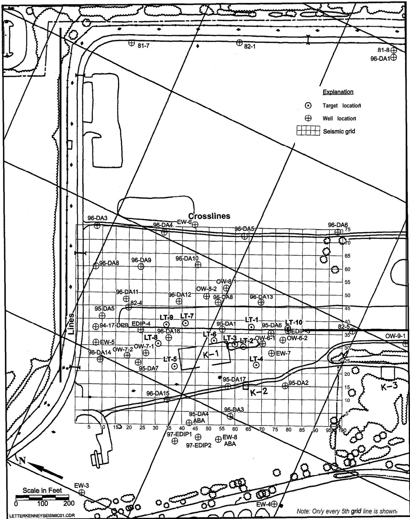
Figure 23. Letterkenny Army Depot Seismic Survey Grid and Target Locations
