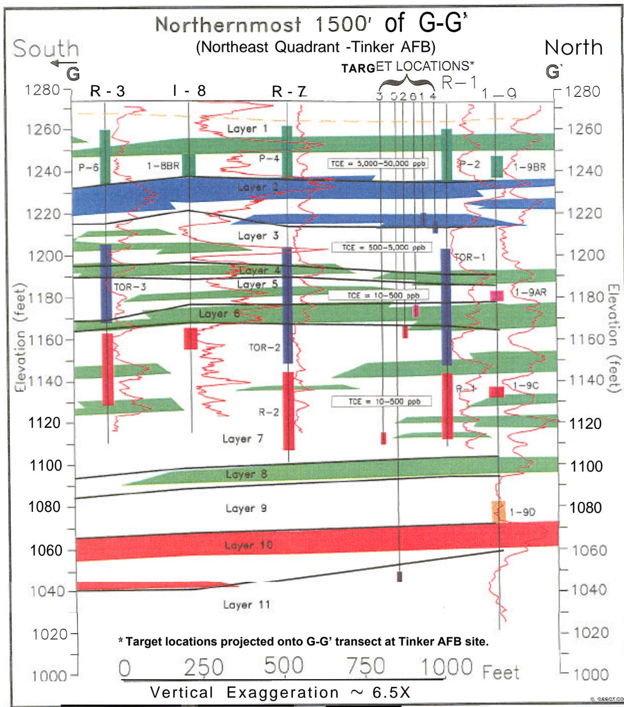
Figure 43. North-South Geologic Cross Section G-6' Showing the Locations and Depths of the Target Wells at Tinker AFB
