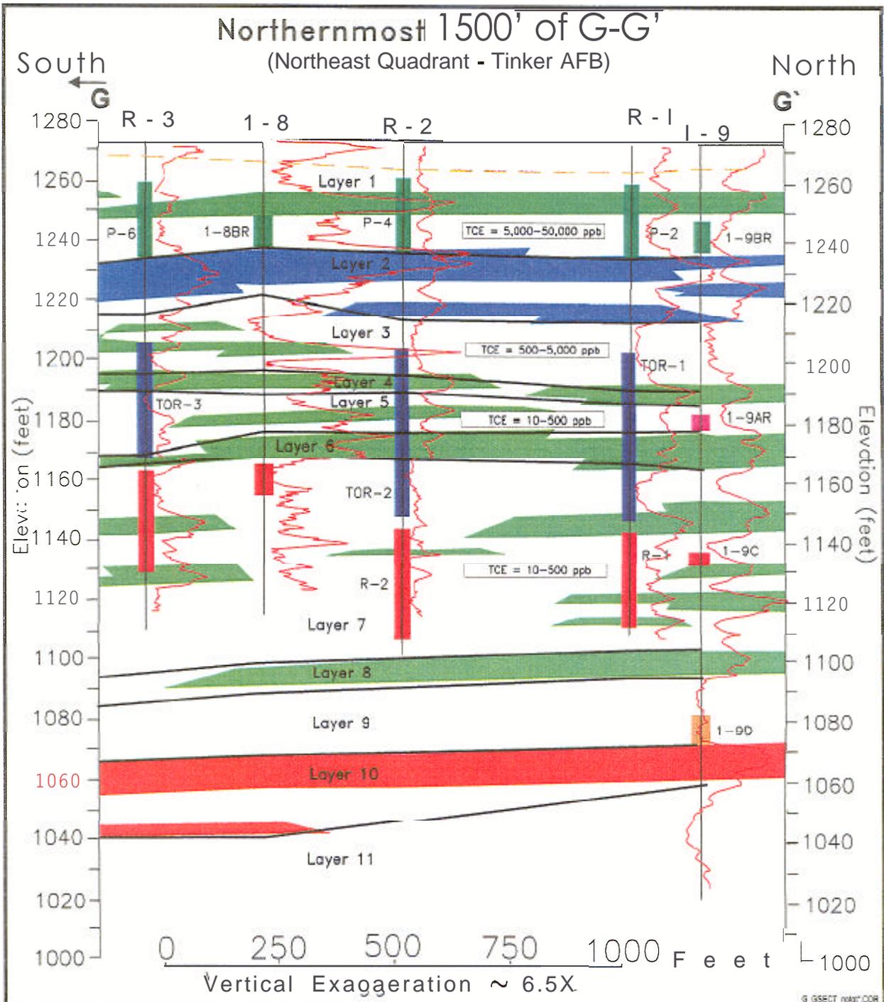
**Figure 16. North-South Geologic Cross Section G-G' at Tinker AFB**
