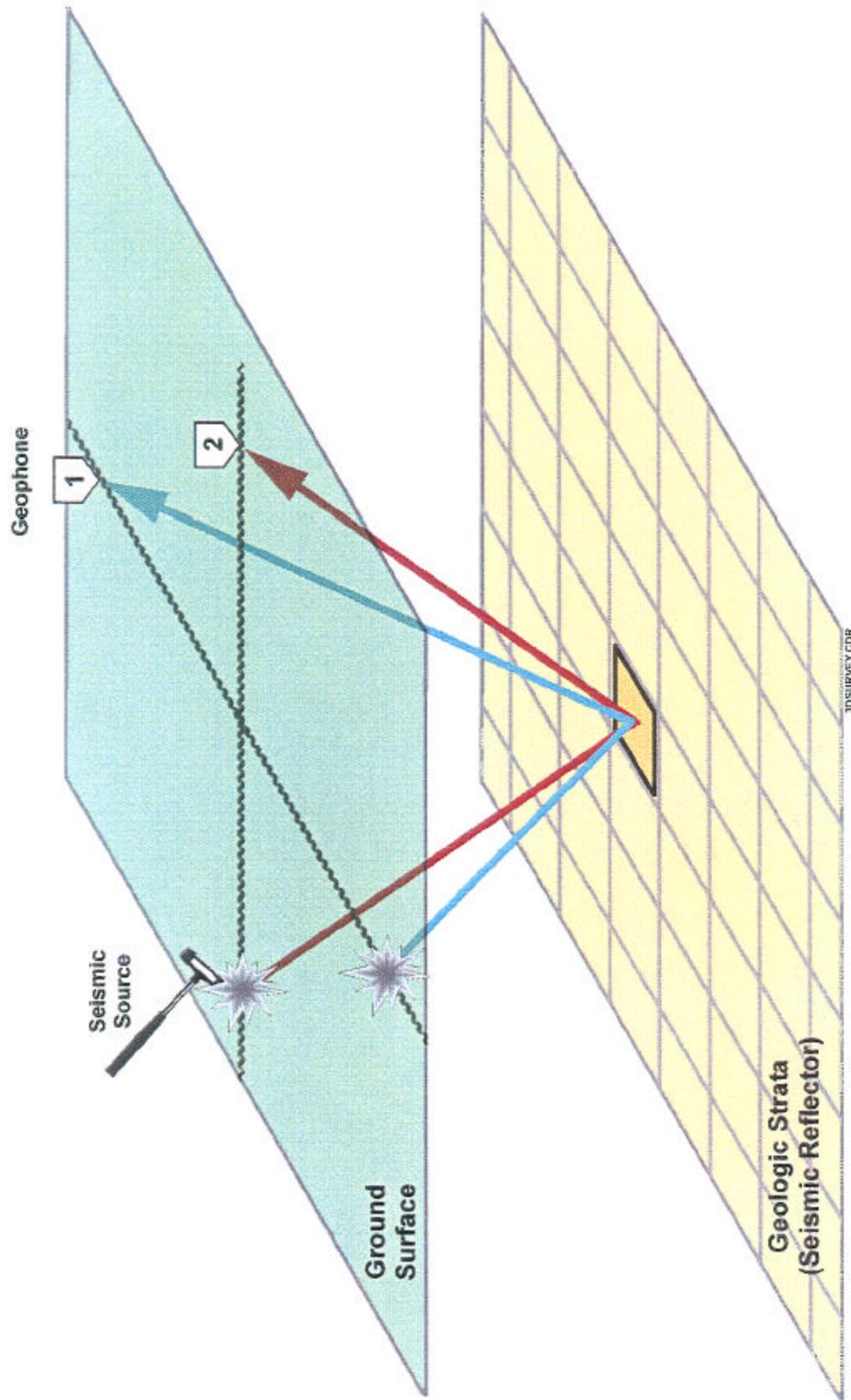
Figure 3. 3-D Seismic Survey
