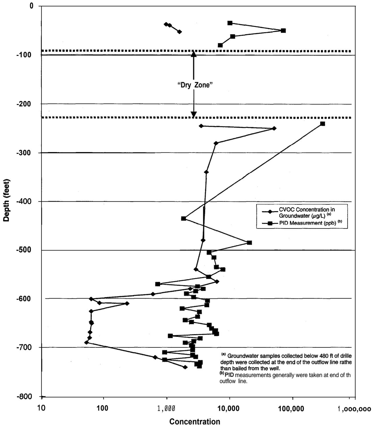
Figure 40. CVOC Concentrations in the Groundwater Along Discrete Sample Depths at Letterkenny Army Depot
