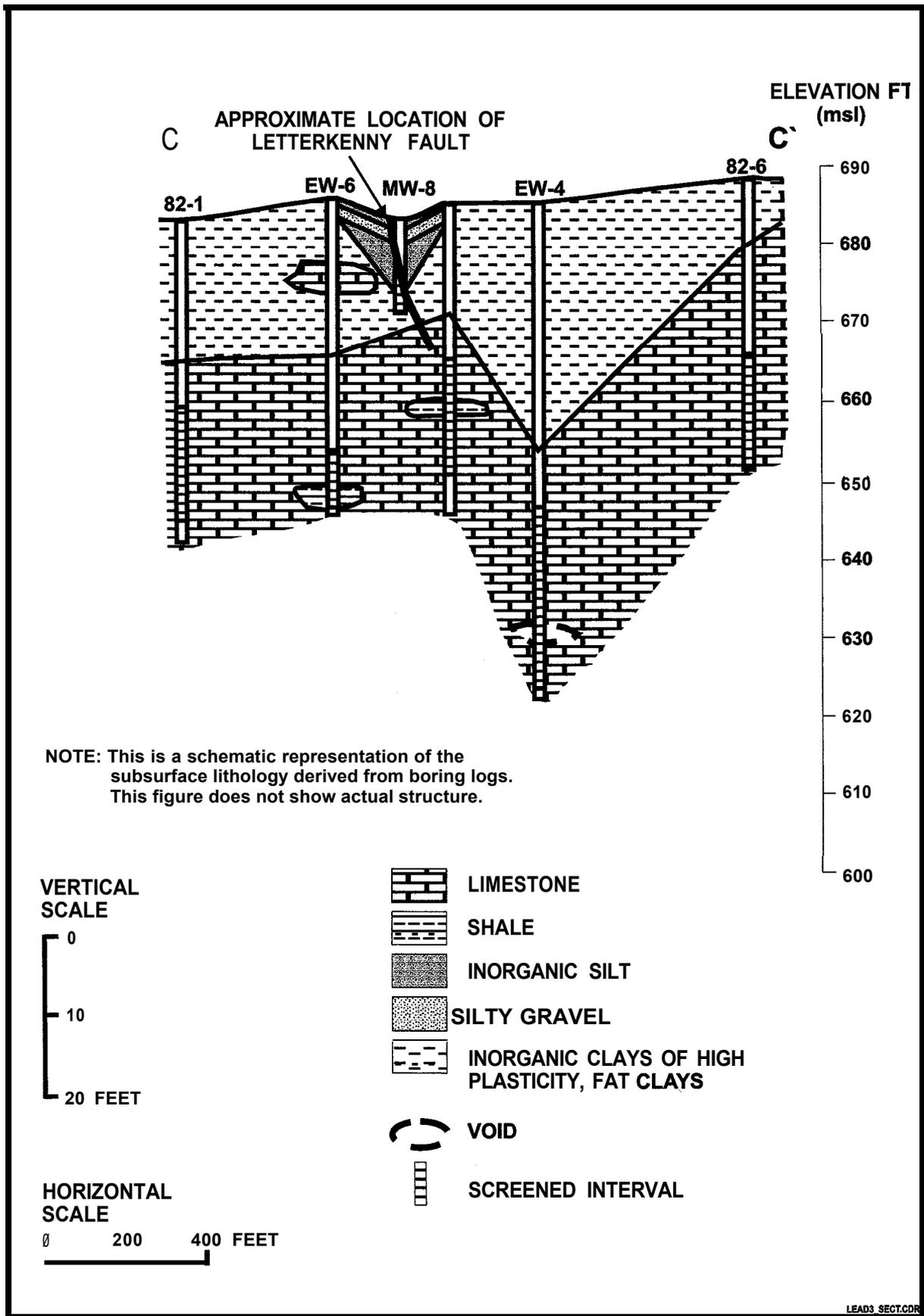
Figure 9. Geologic Cross Section C-C' South of Area K at Letterkenny Army Depot
