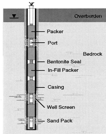
installed and maximizing the number of groundwater zones sampled. The purge volumes necessary for groundwater sampling using the Waterloo System are likely to be smaller than those from conventional nested monitoring wells.
