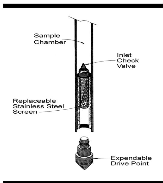
samples if volatilization is not an issue. Finally, as with any single-tube direct-push probe or sampler, there is a potential for cross-contamination between groundwater zones. However this concern can be mitigated by using conductor casings. Floating-layer hydrocarbons may be sampled with a small-diameter bailer lowered through the push rods in one of the Hydropunch™ tools.
