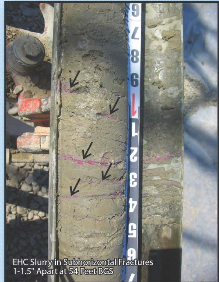
EHC Slurry in Subhorizontal Fractures
