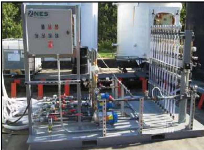
Figure 3: ESTCP Project Permeation Grouting Injection Skid for Injection of Silica Gel Grout
