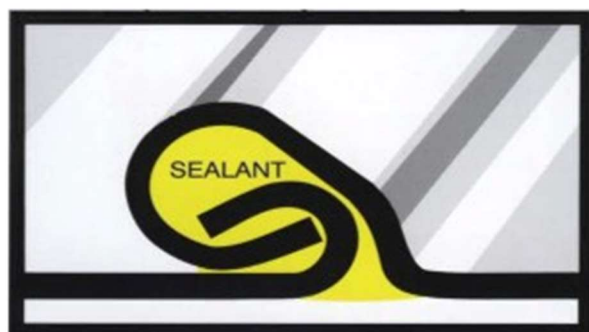
Figure 1: Waterloo Barrier with sealant grout (Waterloo Barriers.com)
