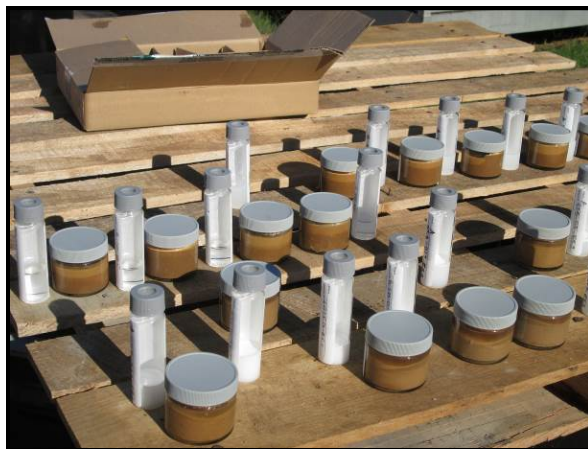
Figure 6.1: On-Site Gel Tests with Site Soils
