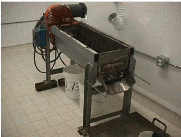
Figure 1. View of pug mill used by ADA Technologies to stabilize mercury waste.
