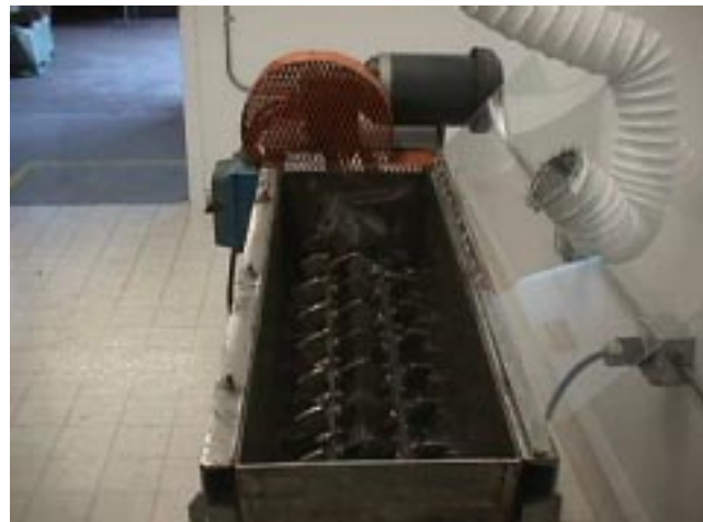
Figure 2. Top view of ADA Technologies' pug mill showing blades, fan, and lid.
