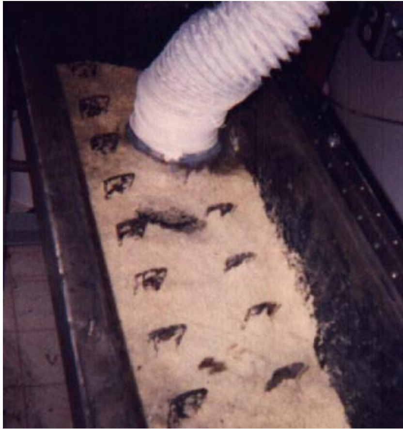
Figure 4. Sulfur in the pug mill before the addition of mercury.
