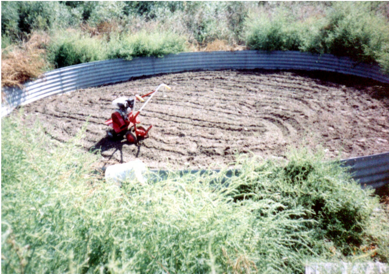
Figure 2. Garden tiller used to till the experimental cells on a biweekly basis
