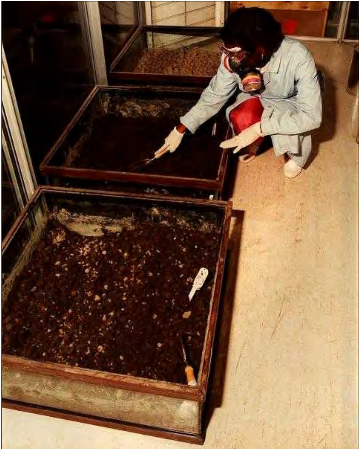
Figure 7. Bench-scale land treatment aquariums
