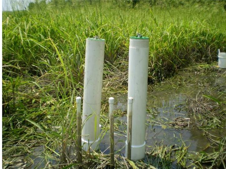
Figure 3-19. *In Situ* Columns IC-3 and IC-4 adjacent to Piezometer Group 1
