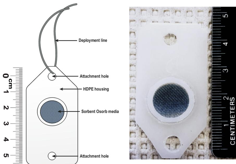
**Figure 1. Schematic (Left) and Photograph (Right) of the PFAS Passive Sampler**
