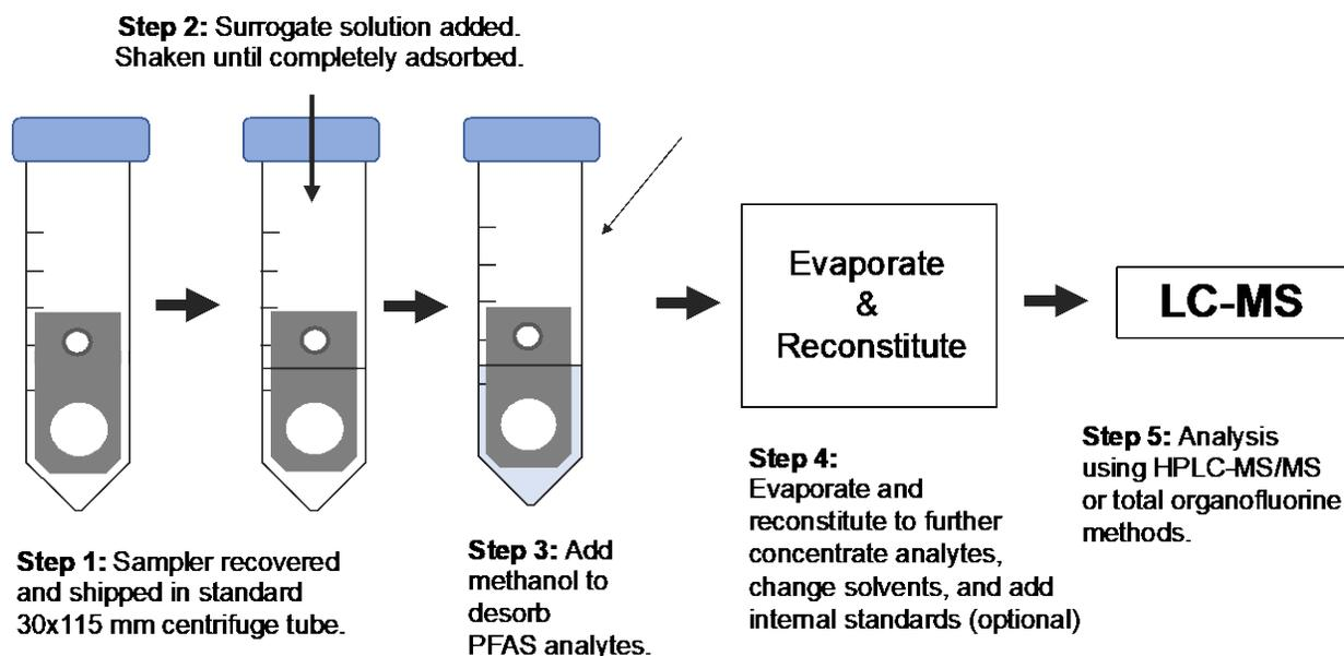
**Figure 4. Diagram of the Extraction Process.**
