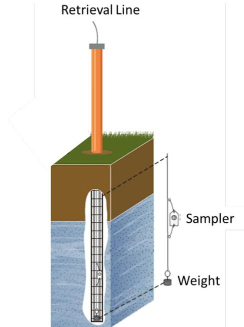
**Figure 2. Depiction of Passive Sampler Deployed in a Groundwater Well.**
