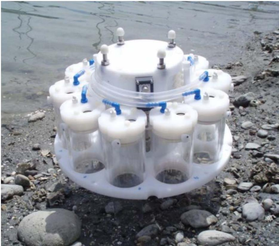
**Figure 23. The SEA Ring Exposure System Used at Pier 7.**
