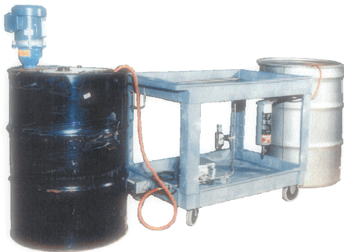
Figure 3. Photo of the apparatus used to test thiol-SAMMS to remove Hg from contaminated vacuum pump oil (treatment was performed in the black 55-gal barrel with the impeller, then the vacuum pump oil was removed, filtered and pumped into the silver receiving barrel).
