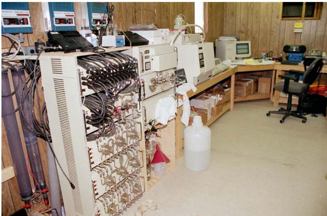
**Fig. 3 Automated sampling and analysis equipment in analytical trailer**
