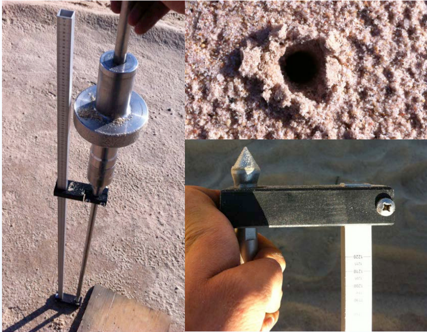
Dynamic Cone Penetrometer (DCP)
