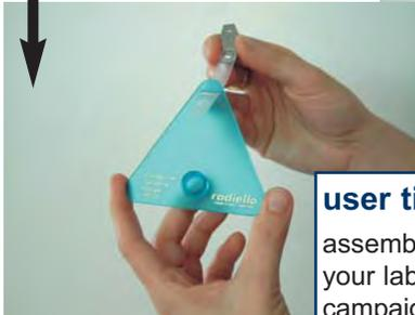
2 ply the strip and insert the peg into the hole
