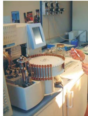
*Usually, the cartridge enters into the Turbomatrix tube by simple pouring. If it does not occur, use a pushing tool to press the cartridge till the nick on the tube.*
