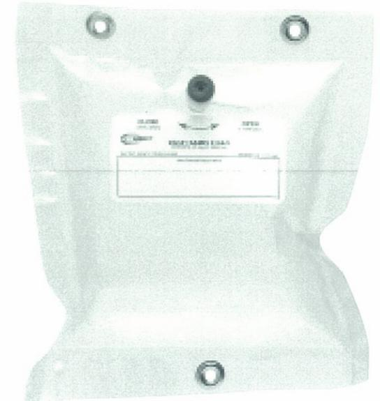
A Tedlar bag is made of two plies of Tedlar film sealed together at the edges and features a valve that allows the interior to be filled. Sample collection requires a pressurized sampling port, a low flow rate pump, or a lung sampler. The bag expands as sample enters. When the target volume of sample is collected, the valve is closed and the Tedlar bag is returned to the laboratory. Air Toxics Ltd. maintains a limited inventory of Tedlar bags in 1 L, 3 L, and 5 L volumes.
