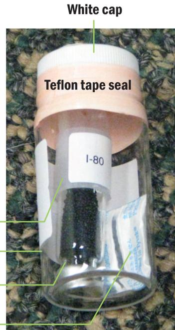
Figure 2: Close-up of WMS™ sampler in its glass overpack shipping vial
