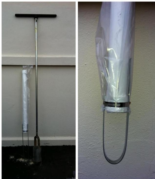
**Figure 24:** Photos of the passive soil vapor probe and hand auger used at NAS JAX
