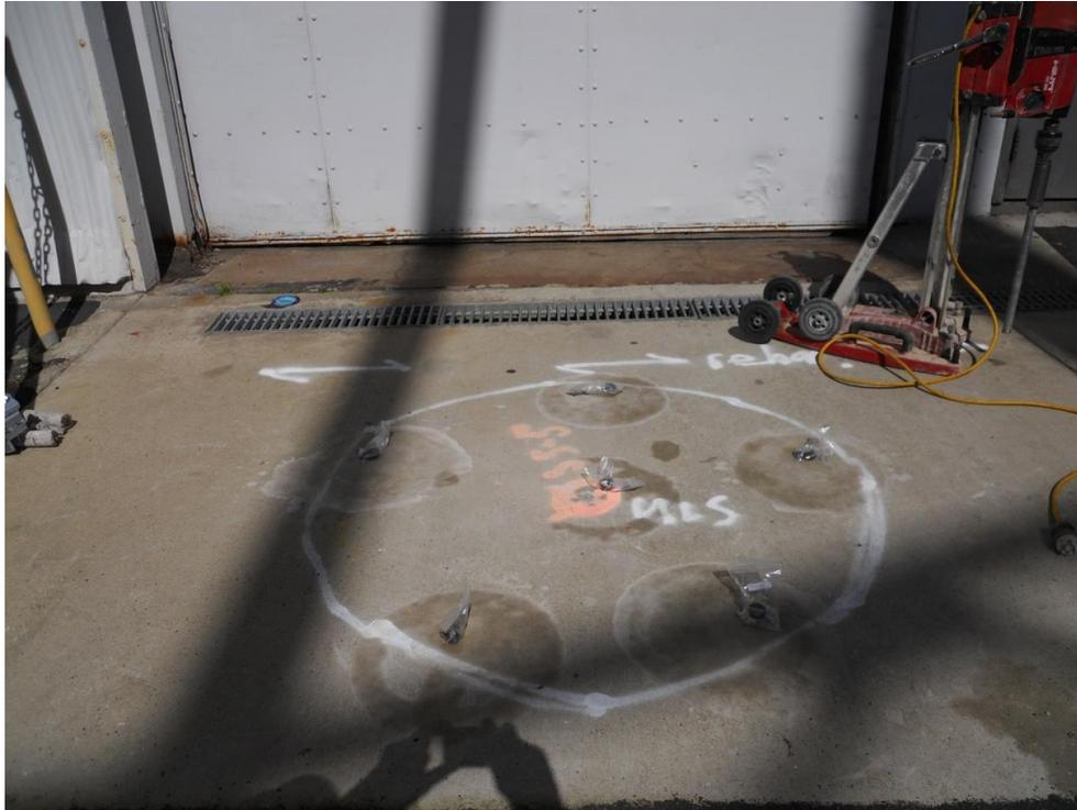
**Figure 18:** Sub-slab probe array (OTC3)
