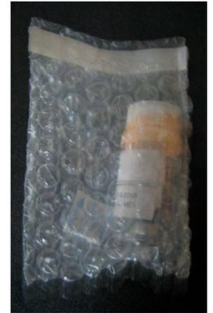
Figure 4: WMS™ Sampler after deployment. Absorbent packet is now in bubble pack, NOT in glass overpack.
