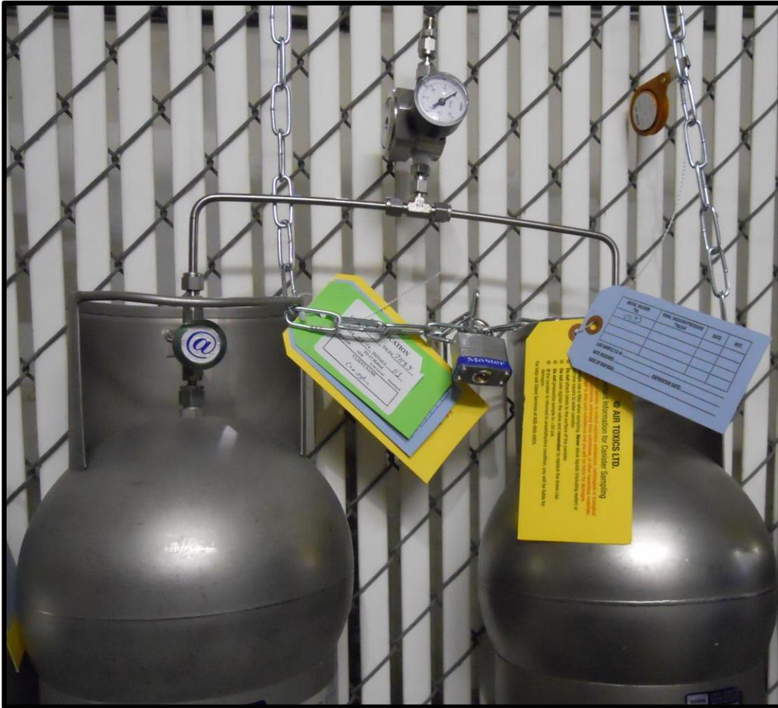
**Figure 2f:** Photo of two 6L Summa canisters and a 3M OVM 3500 sampler (upper right)
