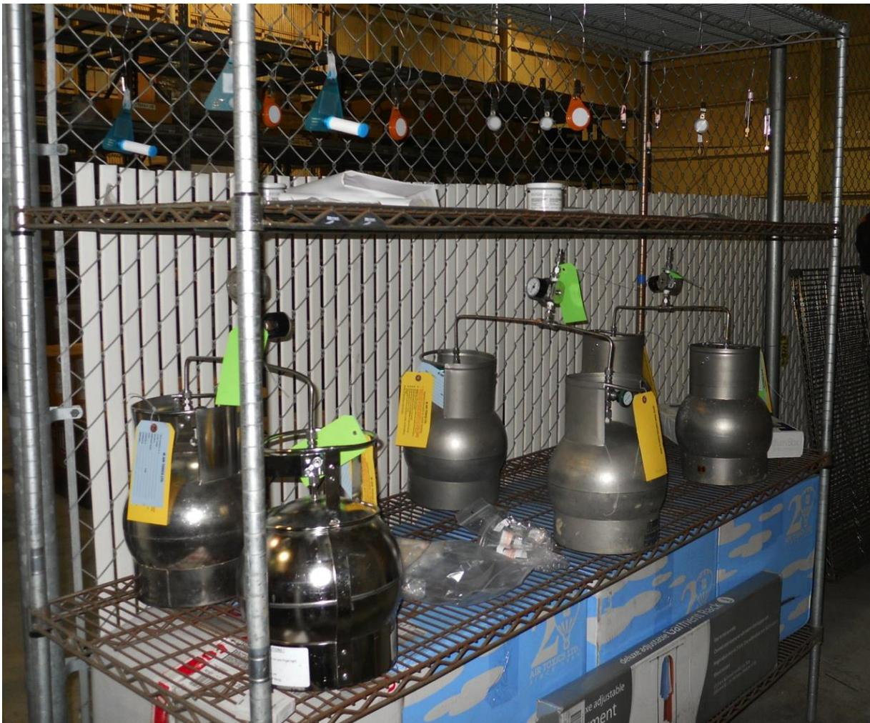
**Figure 15:** Typical layout of indoor air sampling array
