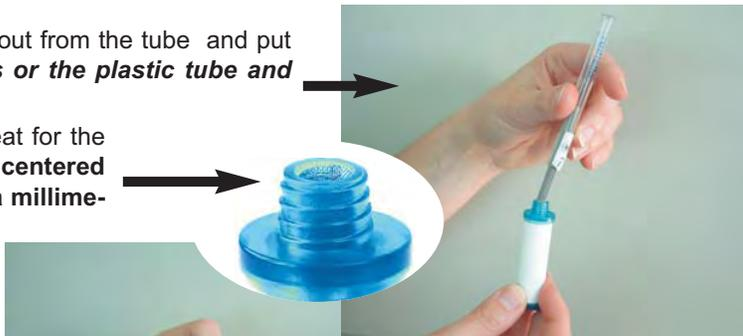
2 keeping the diffusive body in a vertical position, screw it onto the supporting plate
