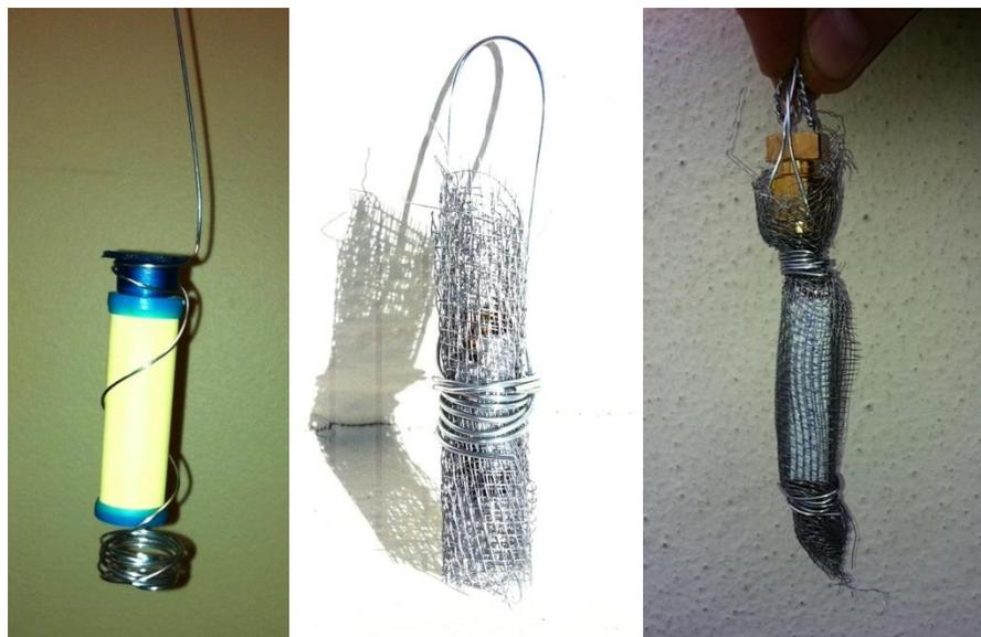
**Figure 26:** Radiello, WMS and ATD Samplers wrapped to protect them from contact with soil
