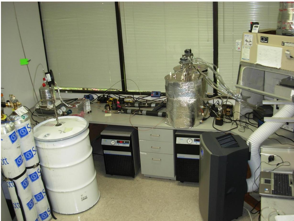
**Figure 12:** Low concentration test apparatus, including (left to right: compressed gas cylinders containing 10 VOCs, drum of activated carbon for purifying dilution air, humidification vessel, mass flow controllers, exposure chambers (covered with insulation), constant temperature bath, and discharge lines to fumehood).
