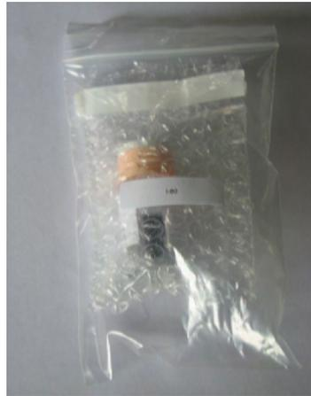
Figure 1: WMS™ sampler with glass overpack vial, unsealed bubble pack and plastic bag.
