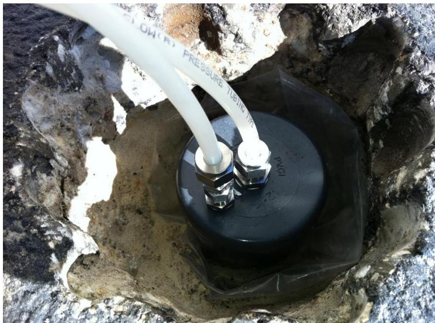
**Figure 25:** Cap of passive soil gas probe at NAS JAX
