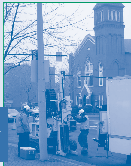
Figure 1. MIP deployment for plume delineation near the former Fannon Petroleum Services site could be completed at each location in less than one hour, with little disruption to ongoing activities.
