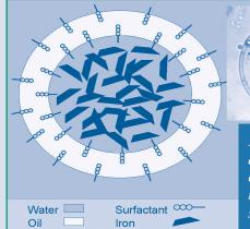
**Figure 1.** EZVI technology demonstrated at the NASA test site employed emulsion droplets containing nanoscale iron particles in water surrounded by an oil-liquid membrane.
