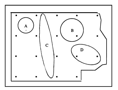
Figure 9.2 Grid Spacing and Ellipse Shape Definitions for the Hot Spot Search Table in Appendix A (Table A. 11)
