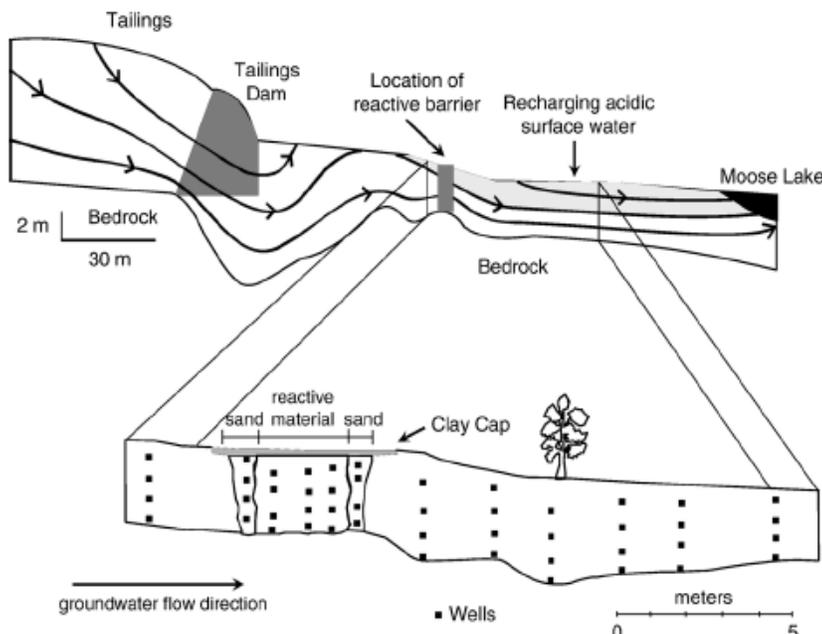
A plume of contaminated ground water continues to flow at an average velocity of 16 m/year. Approximately 50% of the tailings leachate discharges to the surface near the tailings dam, while the remainder flows through the aquifer. Acidic surface water infiltrates the aquifer both up- and down-gradient of the barrier. Approximately 160 m from the tailings dam, the ground water discharges to Moose Lake. (Johnson et al., 2000; Figure 8)
