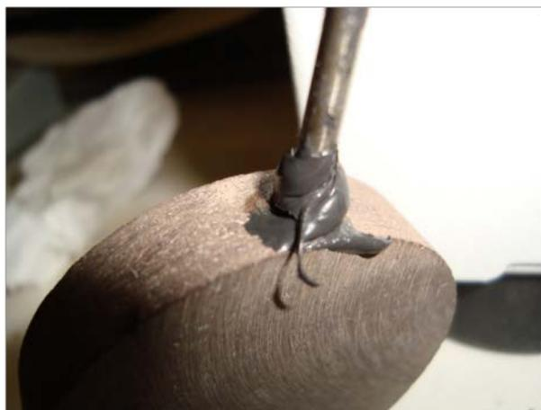
**Figure 1 – Photograph of the temperature monitoring disc for red mudstone with a thermocouple placed inside the drilled hole to monitor the temperature profile in the disc during the heating tests.**
