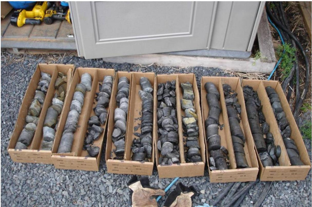
**Figure 5.29. Pre-Treatment Rock Cores**
