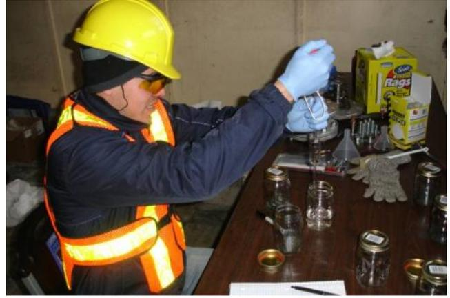
**Figure 5.28. Cutting and Methanol Preservation of the Cores**
