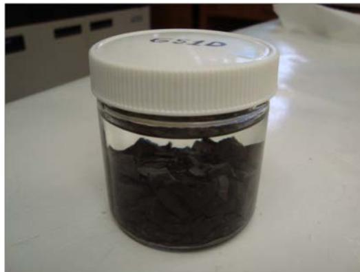
**Figure 5 – Photograph of the 125mL jar containing the TCE extract from grey mudstone.**
