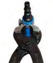
To remove a Stepless Ear Clamp, grasp the strip end with the pincer and pull it away
