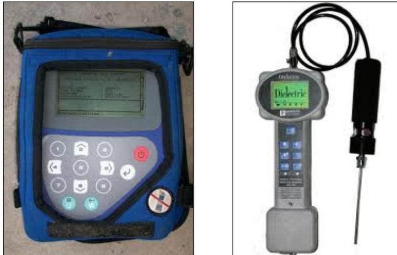
**Figure 28:** Vapor monitoring equipment: GEM2000 Landfill Gas Monitor (left) and Dielectric MGD-2002 Helium & Hydrogen Detector (Right)
