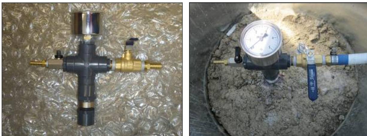
**Figure 27:** Injection wellhead design
