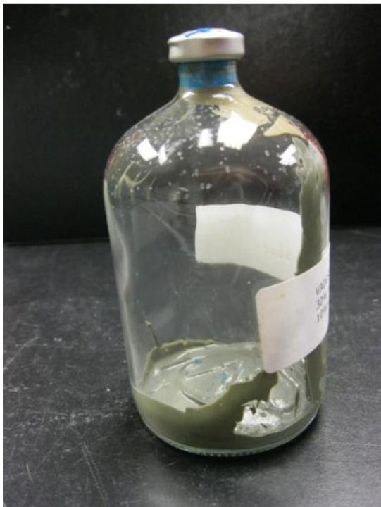
**Figure 2-2:** Microcosm Bottle with Soil at 30 Percent Moisture
