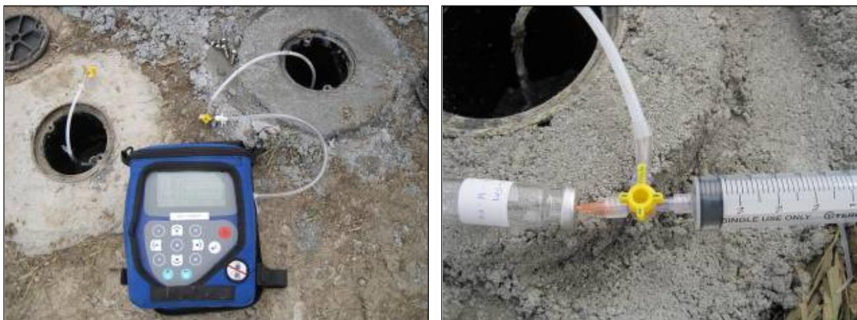
**Figure 21:** GEM2000 readings and vapor sampling
