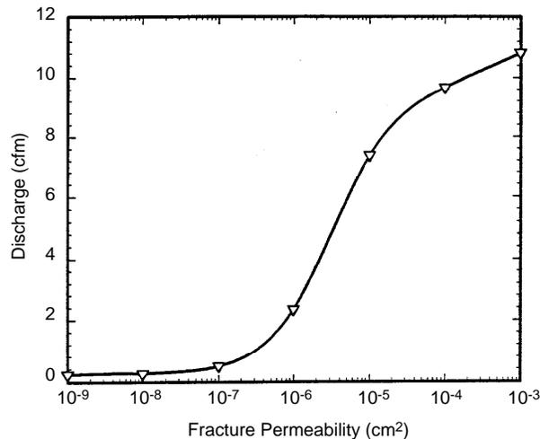
Figure 3-8. Air discharge from a well intersecting a flat-lying circular fracture as a function of the permeability of the fracture. (Formation permeability is  $10^{-9}$  cm<sup>2</sup>.)
