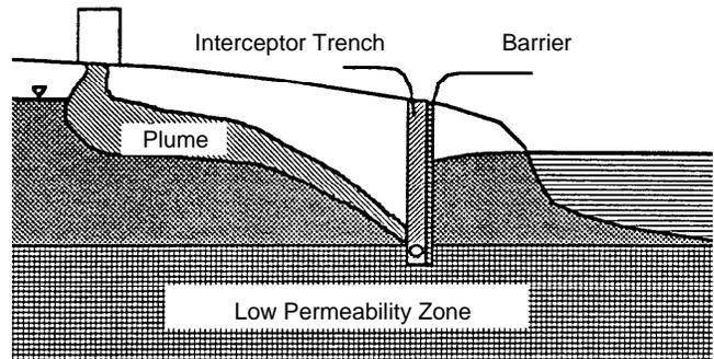
Figure 4-11. Interceptor trench coupled with a hydraulic barrier to minimize recharge from an adjacent surface waterbody.
