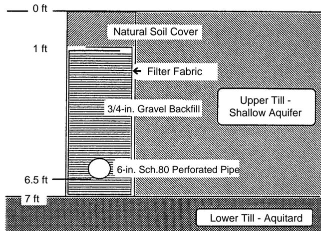
Figure 4-25. Schematic cross section of trench construction (38).
