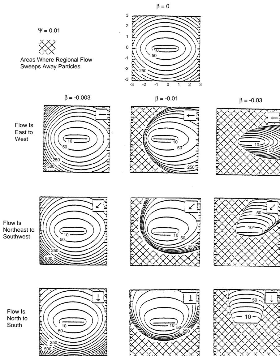
Figure 4-8. Dimensionless arrival times as a function of location for various strengths and directions of regional flow (11).
