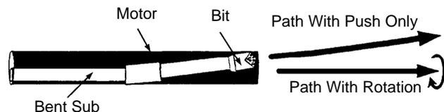
**Figure 2-4. Directional drilling with a downhole motor.**
