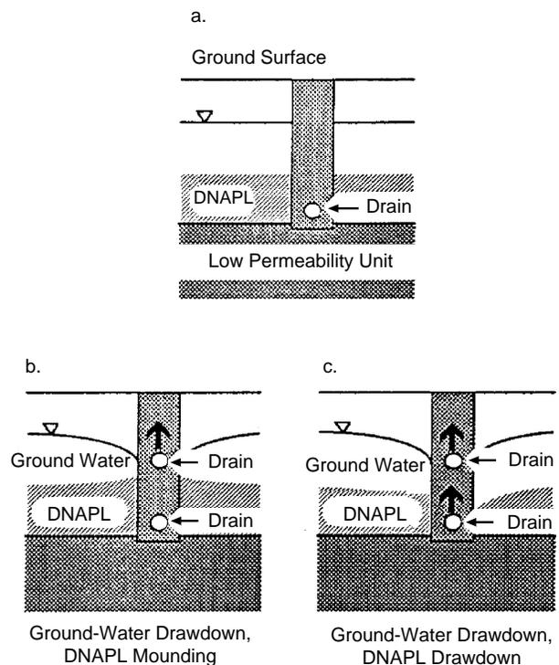
Figure 4-13. Trench systems for DNAPL recovery: a) one-drain system, b) two-drain system with upper drain pumping, and c) two-drain system with both drains pumping (22).
