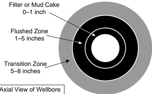
Figure 2-5. Potential damaged zones around a horizontal wellbore.
