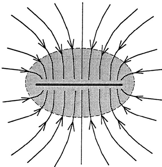
Figure 2-11. Flow paths to a horizontal well in a thin aquifer with no regional flow. Lines are nearly straight and parallel within the patterned area.
