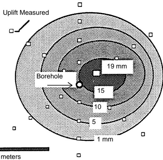
Figure 3-3. Typical pattern of uplift over a shallow, gently dipping hydraulic or pneumatic fracture.
