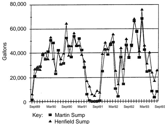
Figure 4-26. Monthly extraction from interceptor trench sumps.
