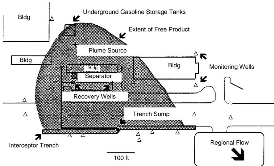
Figure 4-16. Plan of the Westminster gasoline recovery site (15).
