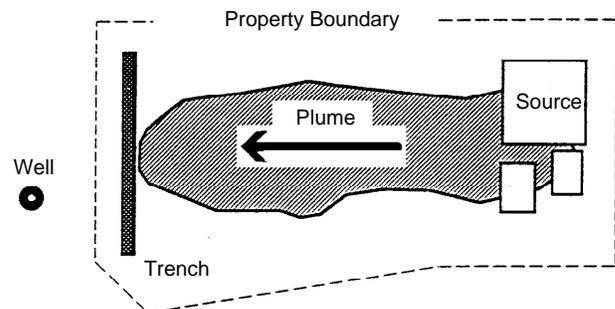
Figure 4-12. Trench used to capture plume and prevent migration to an offsite well.
