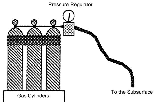
Figure 3-4. Aboveground equipment used for pneumatic fracturing (9).
