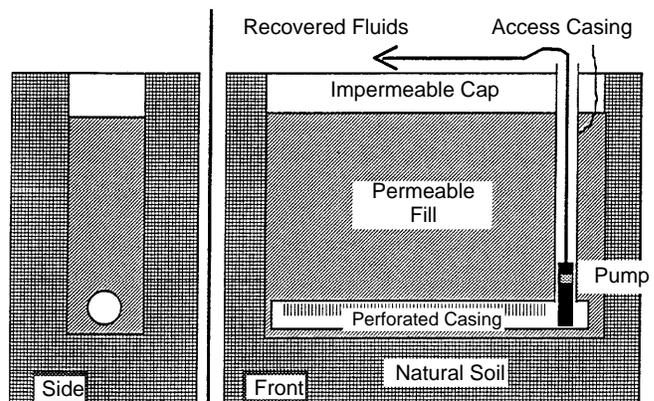
Figure 4-1. Cross sections of a basic interceptor trench configuration showing permeable backfill and perforated casing.
