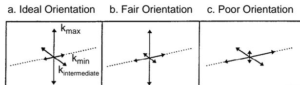
Figure 2-14. Orientations of horizontal well (dashed line) relative to principal directions of permeability.
