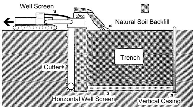
Figure 4-2. Schematic of continuous excavation and completion technique (6).
