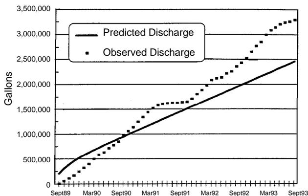
Figure 4-27. Observed and predicted discharges from trench system.
