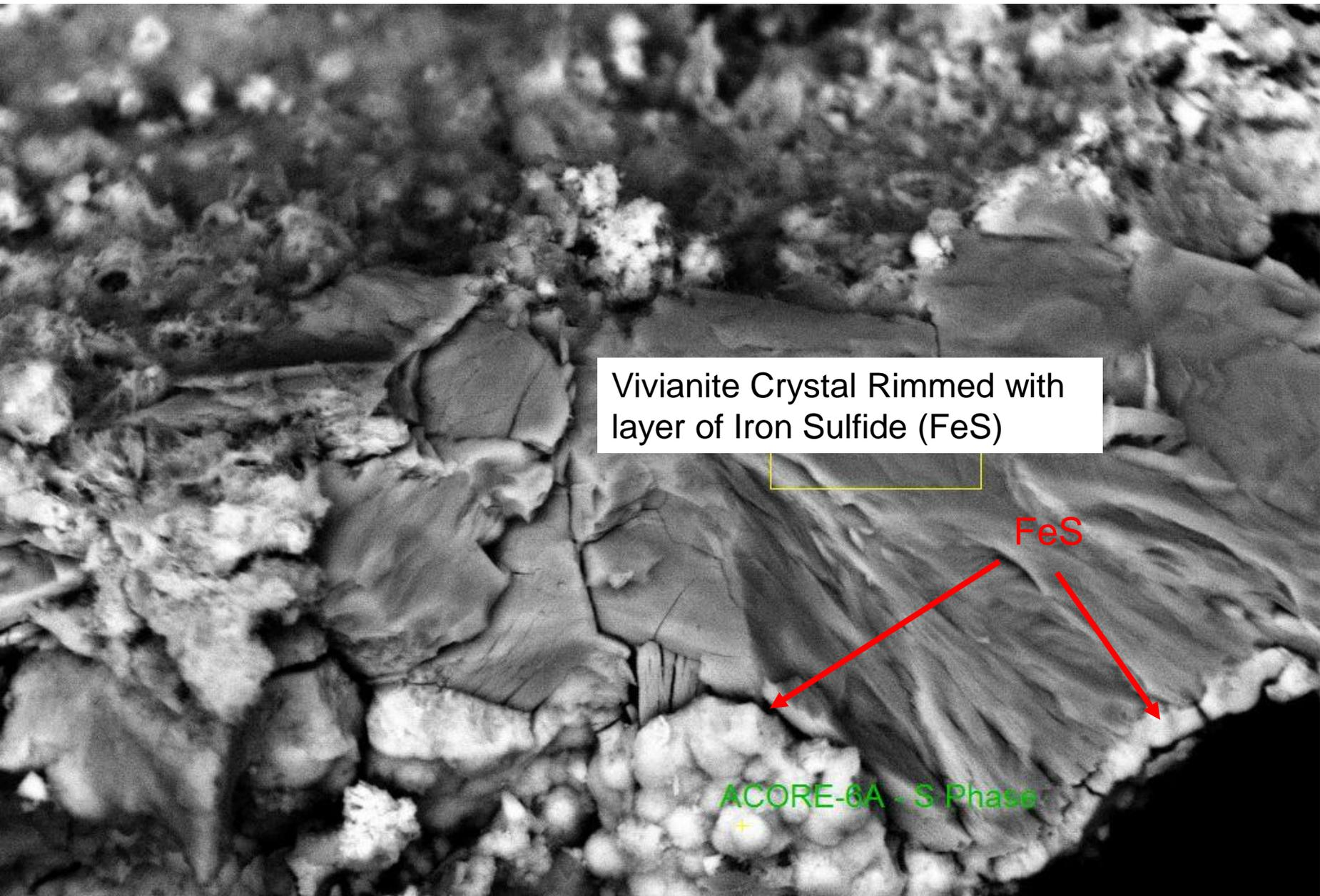
Vivianite Crystal Rimmed with layer of Iron Sulfide (FeS)
