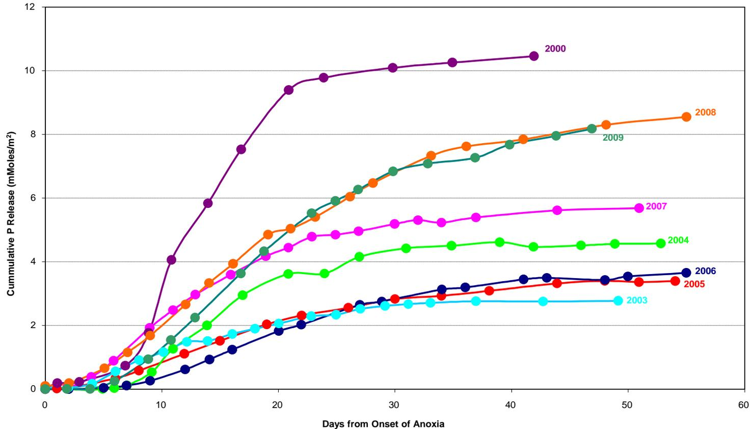
Laboratory tests of 2008 pond sediment core samples produced the highest release of phosphorus observed since the alum treatment.
