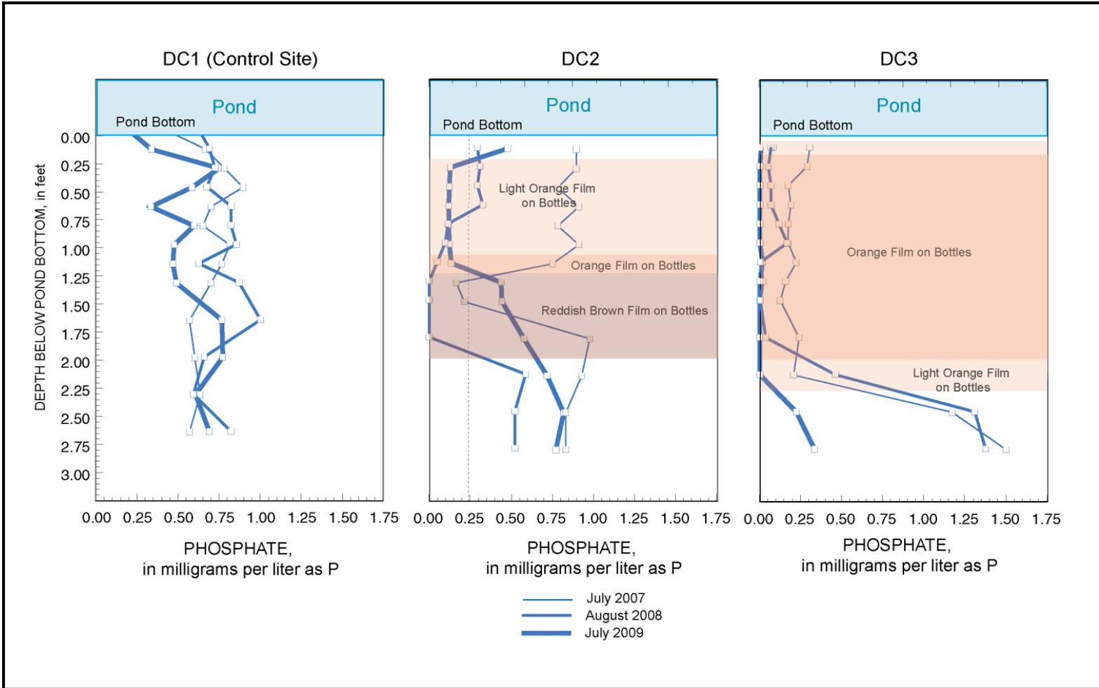
Phosphate Concentration Profiles from Pond-Bottom Vertical Diffusion Chambers (DCs) at 3, 4, and 5 years after PRB Installation
