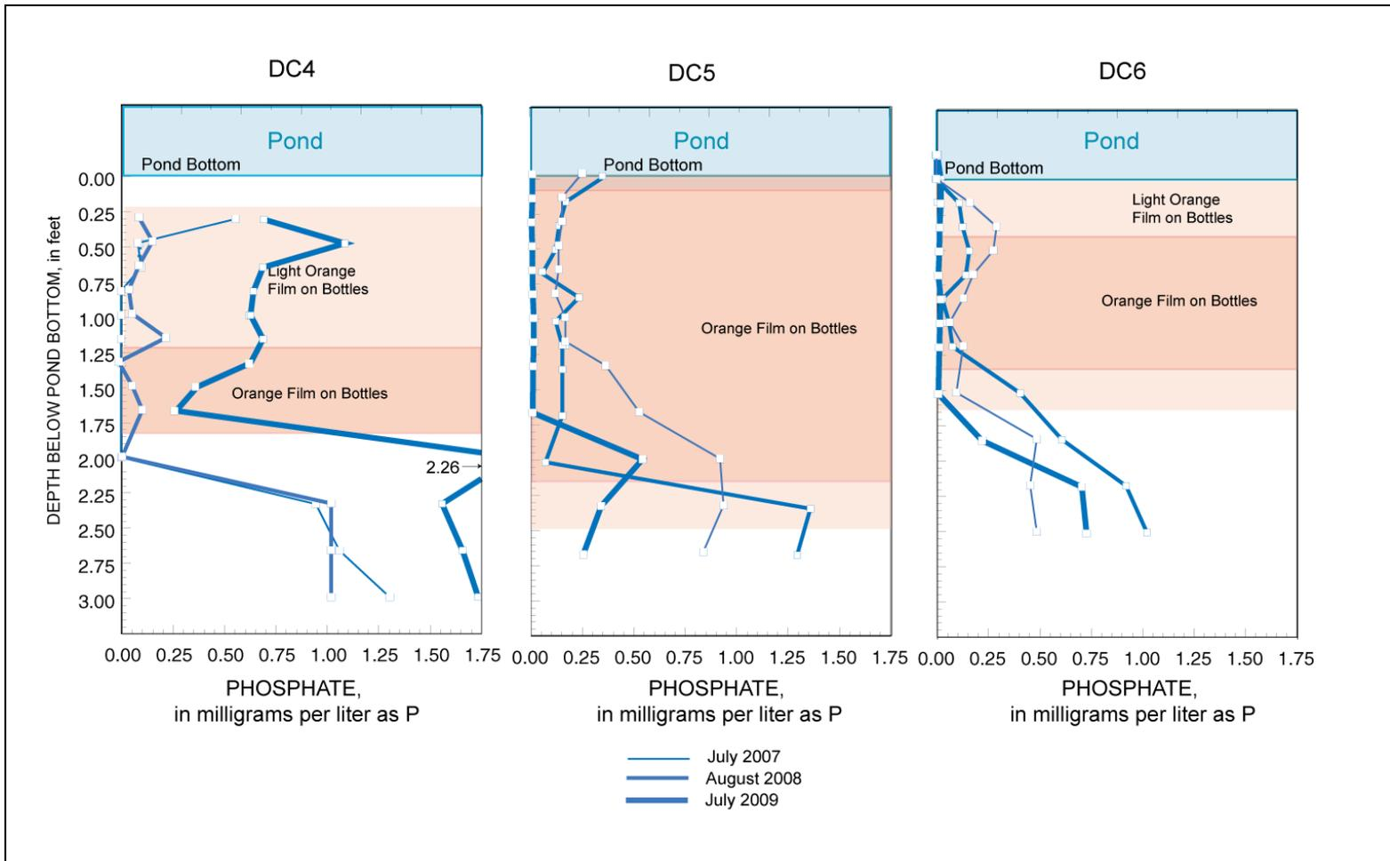
Phosphate Concentration Profiles from Pond-Bottom Vertical Diffusion Chambers (DCs) at 3, 4, and 5 years after PRB Installation
