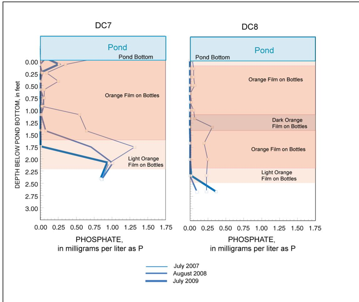
Phosphate Concentration Profiles from Pond-Bottom Vertical Diffusion Chambers (DCs) at 3, 4, and 5 years after PRB Installation
