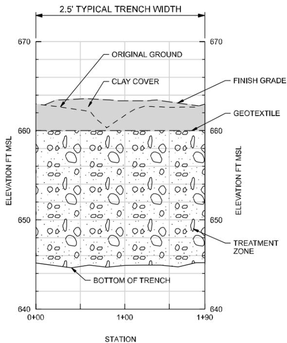
**BIOWALL S-3B CONSTRUCTED PROFILE**
