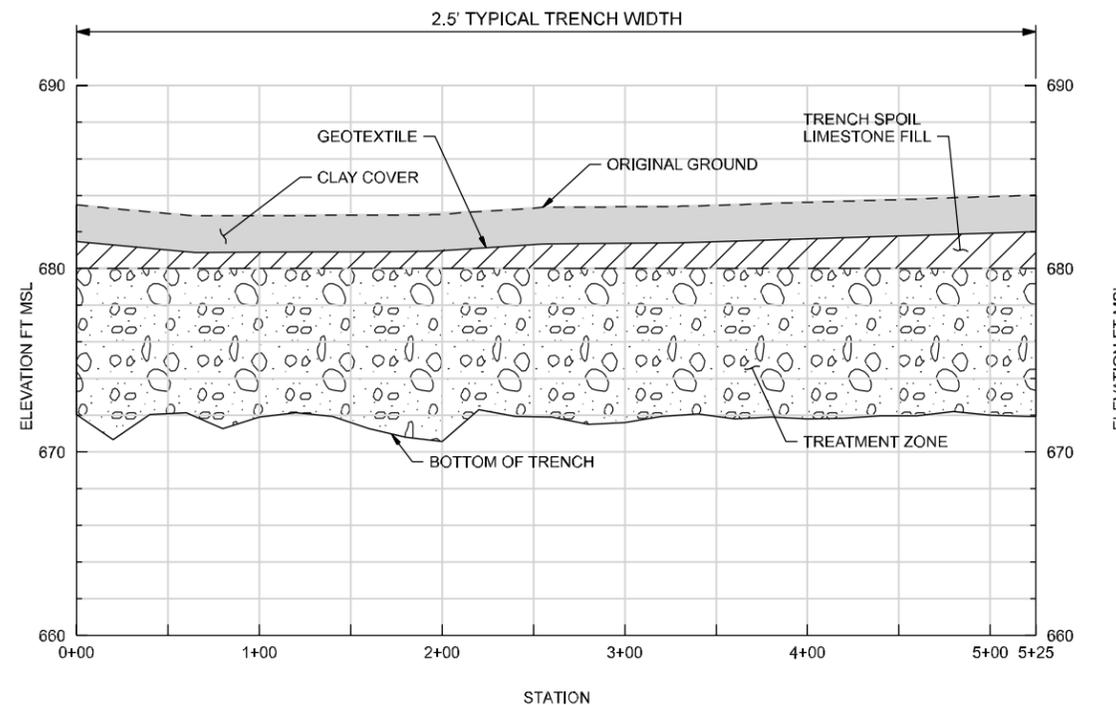
**BIOWALL S-2 CONSTRUCTED PROFILE**
