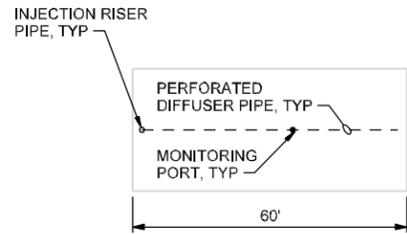
**BIOWALL M-1B PIPING LAYOUT**
