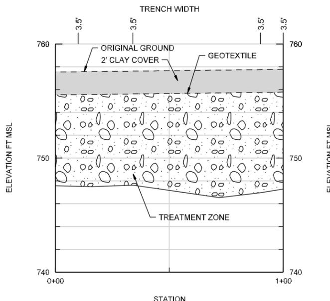
**BIOWALL M-6 CONSTRUCTED PROFILE**
