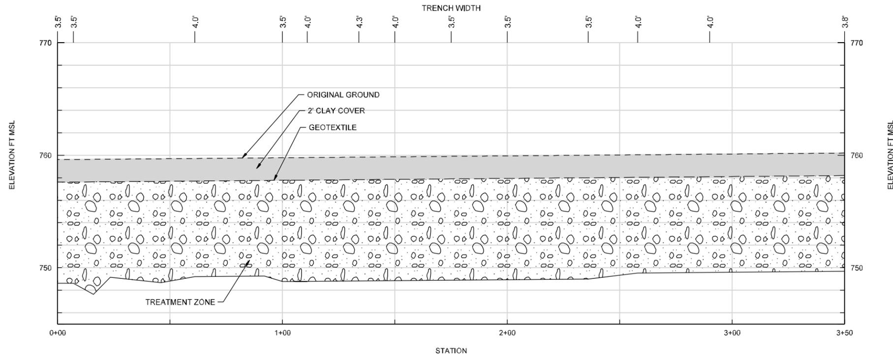
**BIOWALL M-3 CONSTRUCTED PROFILE**
