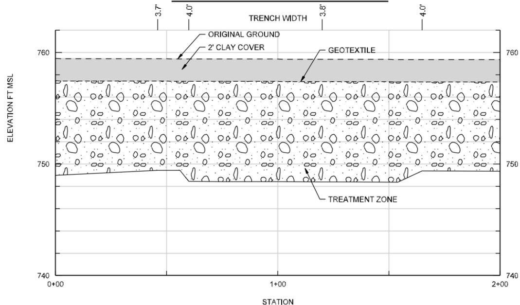
**BIOWALL M-2 CONSTRUCTED PROFILE**
