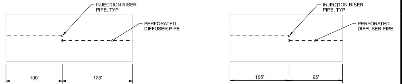
**BIOWALL S-3A AND S-3C PIPING LAYOUT**
