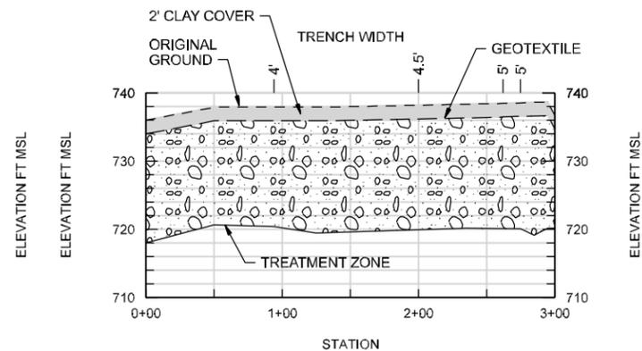
**BIOWALL F-6B CONSTRUCTED PROFILE**
