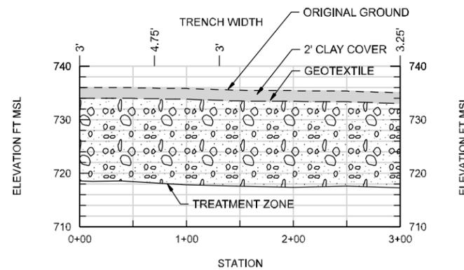
**BIOWALL F-8B CONSTRUCTED PROFILE**
