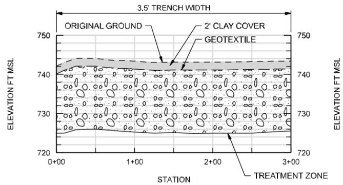
**BIOWALL F-4B CONSTRUCTED PROFILE**
