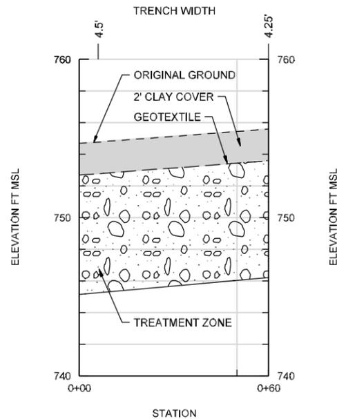
**BIOWALL M-1B CONSTRUCTED PROFILE**
