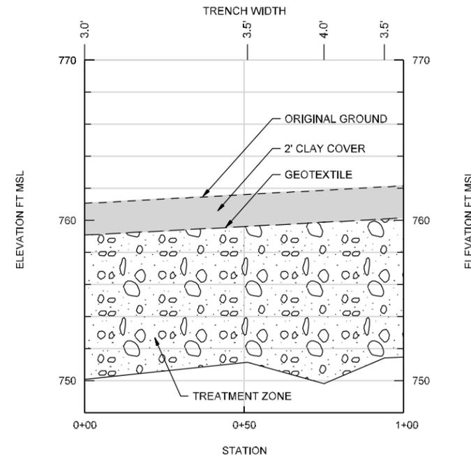
**BIOWALL M-4 CONSTRUCTED PROFILE**
