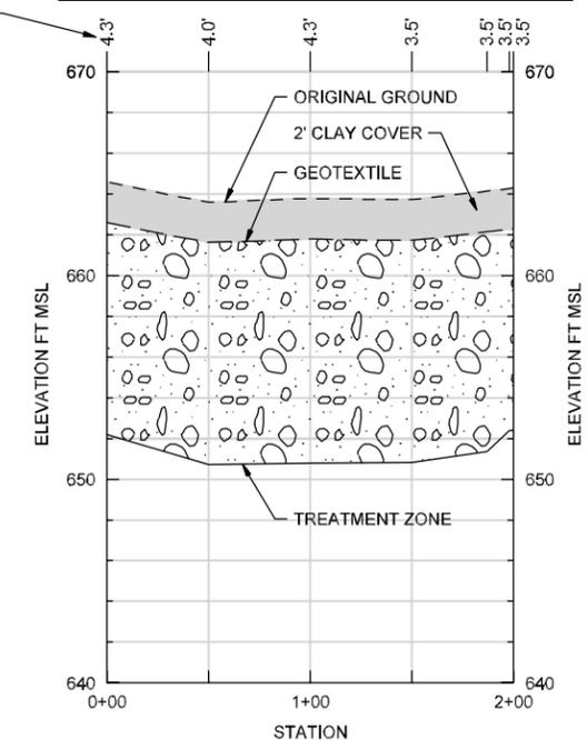
BIOWALL S-3E CONSTRUCTED PROFILE
