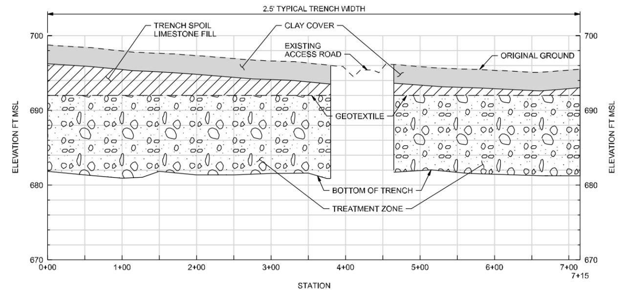
**BIOWALL S-1 CONSTRUCTED PROFILE**
