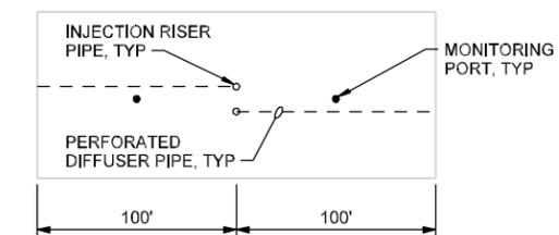
BIOWALL S-3E PIPING LAYOUT
