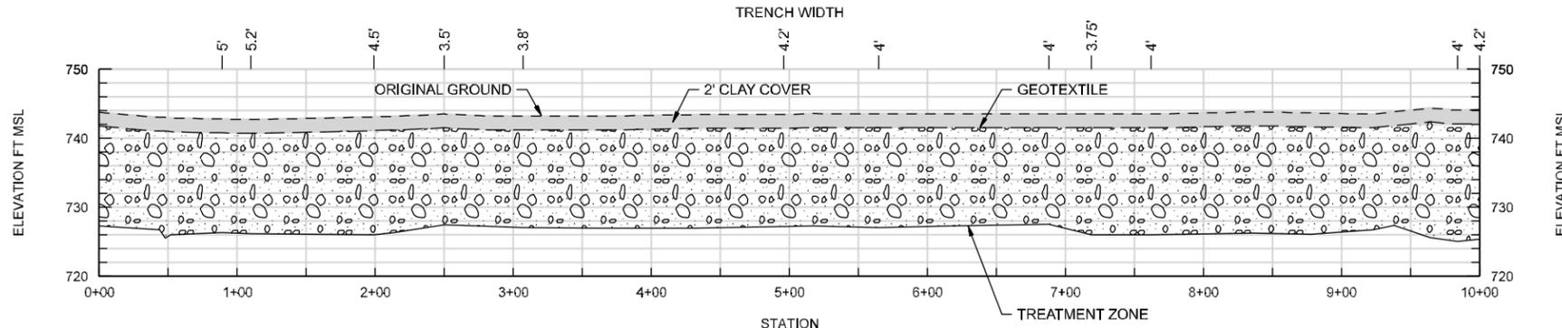
**BIOWALL F-5 CONSTRUCTED PROFILE**
