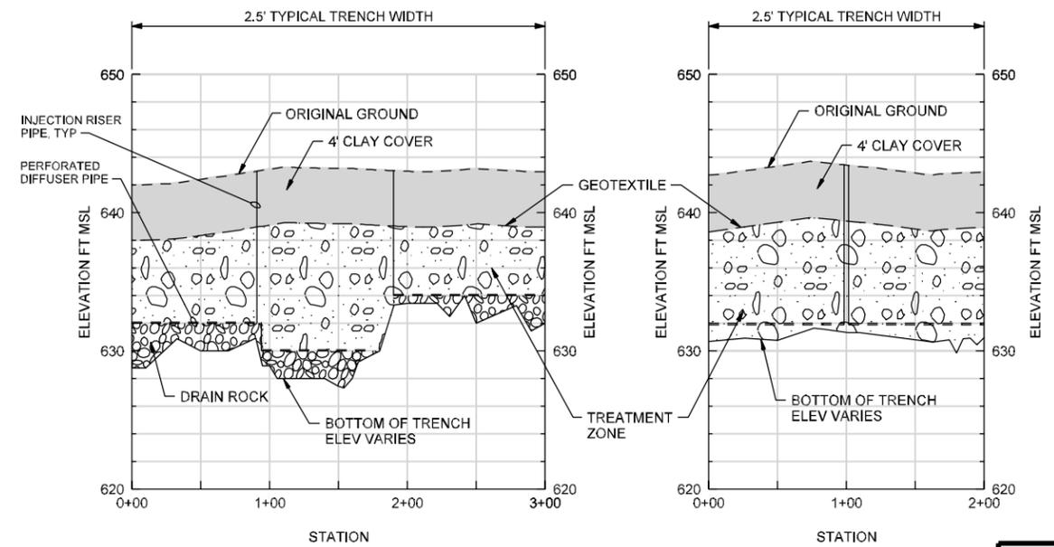
**BIOWALL S-5 CONSTRUCTED PROFILE**
