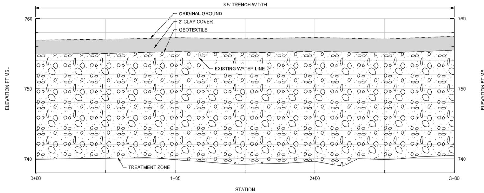
**BIOWALL E-1 CONSTRUCTED PROFILE**
