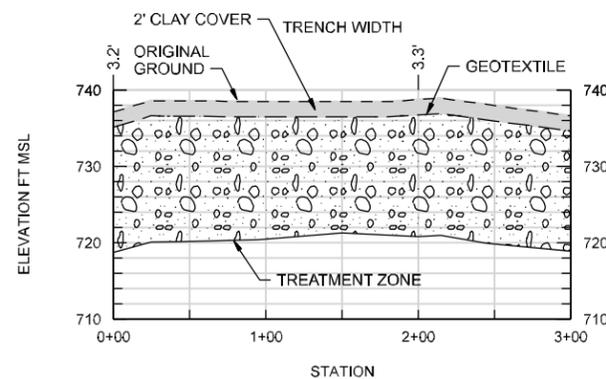
**BIOWALL F-6A CONSTRUCTED PROFILE**
