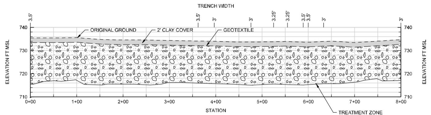
**BIOWALL F-2 CONSTRUCTED PROFILE**
