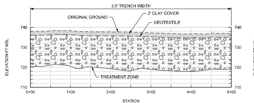
**BIOWALL F-7 CONSTRUCTED PROFILE**
