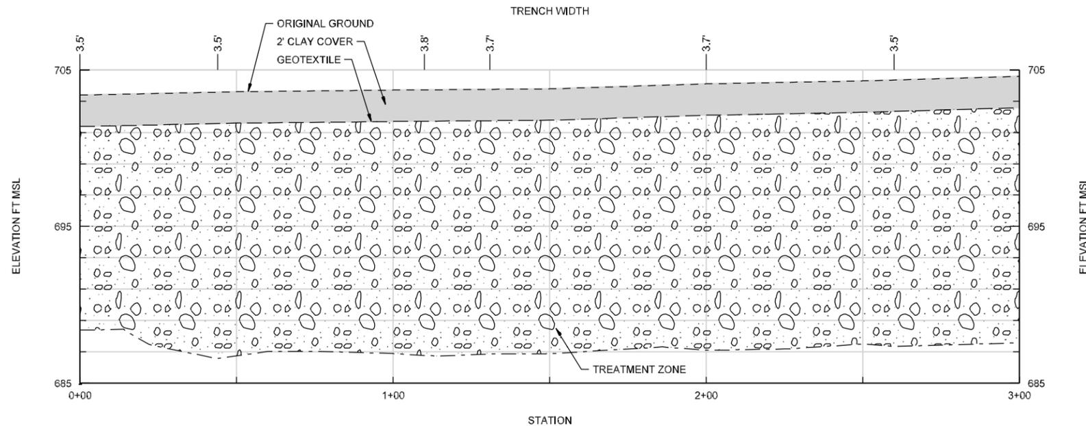
**BIOWALL S-8 CONSTRUCTED PROFILE**
