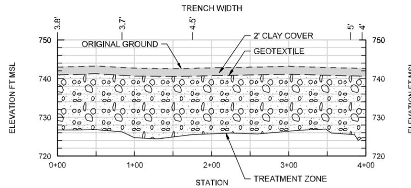
**BIOWALL F-4C CONSTRUCTED PROFILE**
