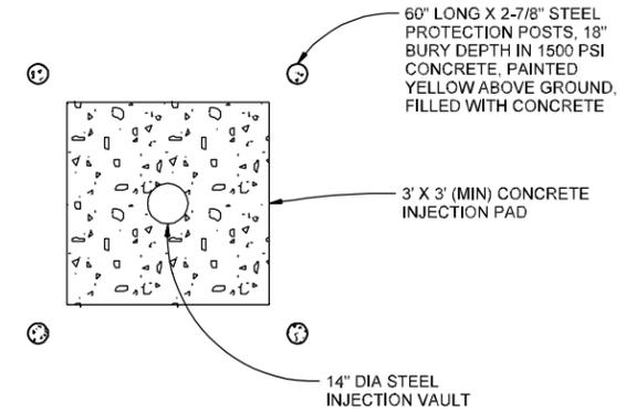
**BOLLARD INSTALLATION DETAIL**
