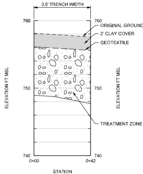
**BIOWALL M-1A CONSTRUCTED PROFILE**
