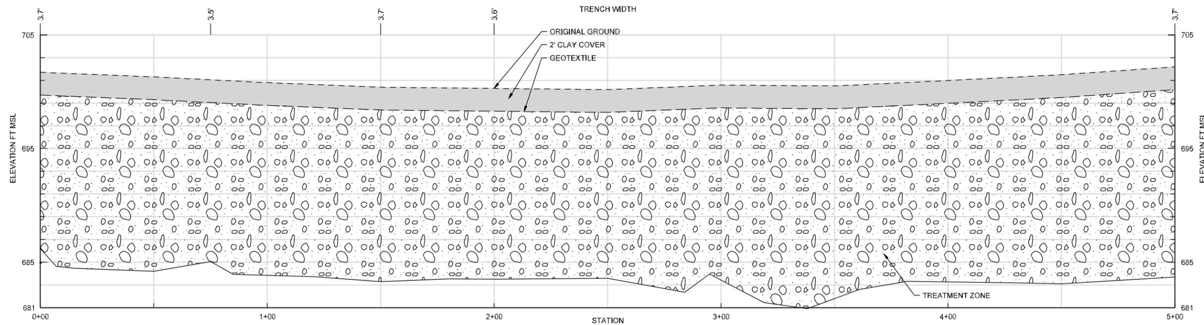
**BIOWALL S-9 CONSTRUCTED PROFILE**
