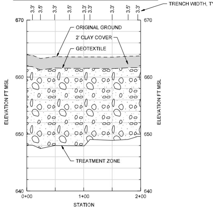
BIOWALL S-3D CONSTRUCTED PROFILE
