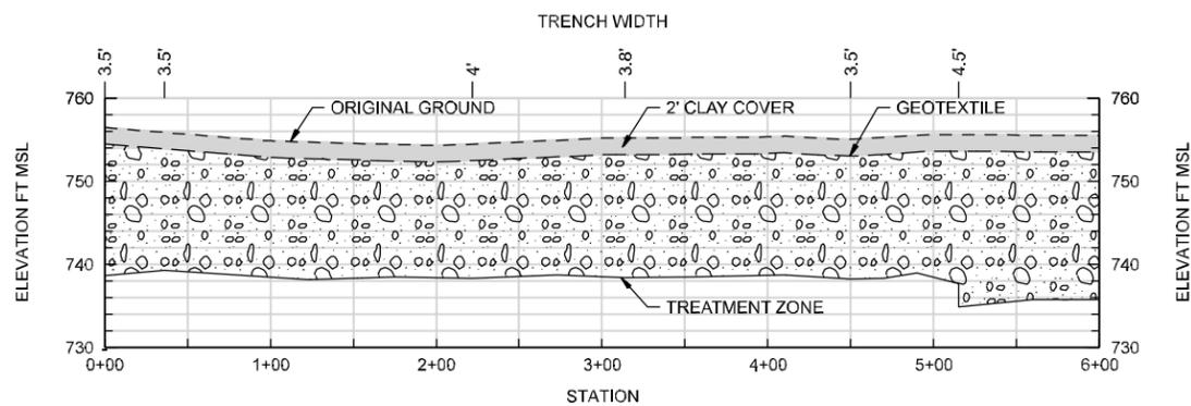
**BIOWALL F-1 CONSTRUCTED PROFILE**
