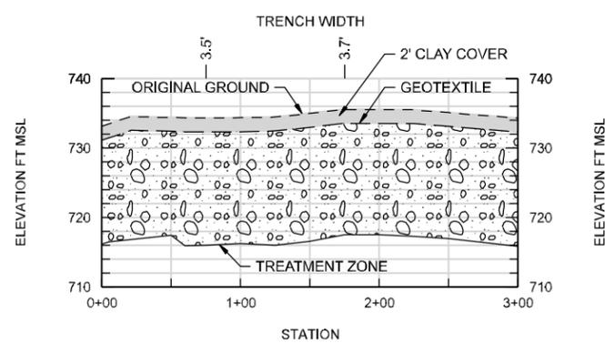
**BIOWALL F-8A CONSTRUCTED PROFILE**
