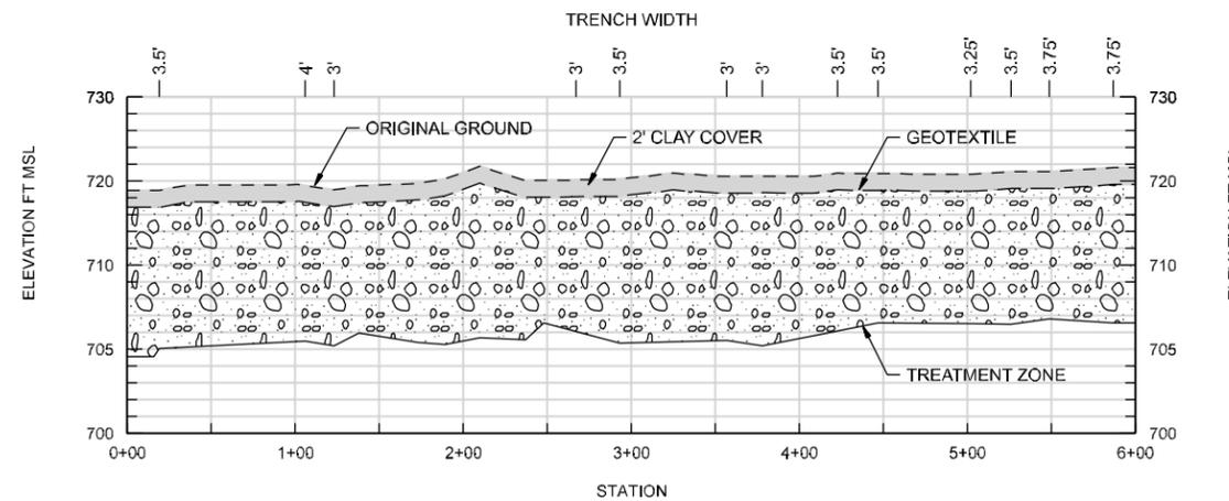
**BIOWALL F-3B CONSTRUCTED PROFILE**
