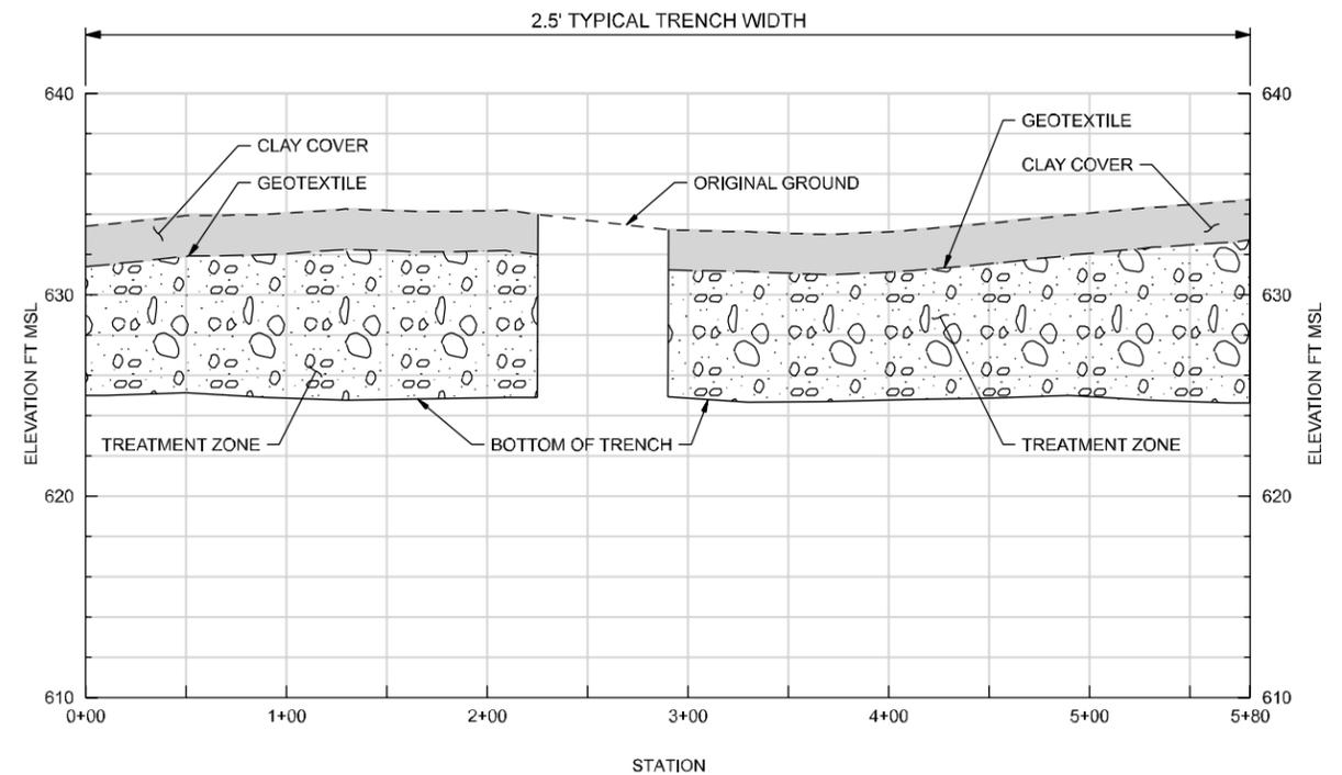
**BIOWALL S-6 CONSTRUCTED PROFILE**
