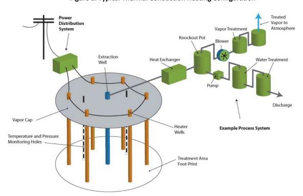
Figure 2. Typical Thermal Conduction Heating Configuration
