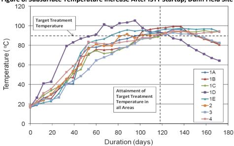
Figure 8. Subsurface Temperature Increase After ISTT Startup, Dunn Field Site
