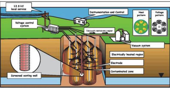
Figure 1. Typical ERH System Configuration
