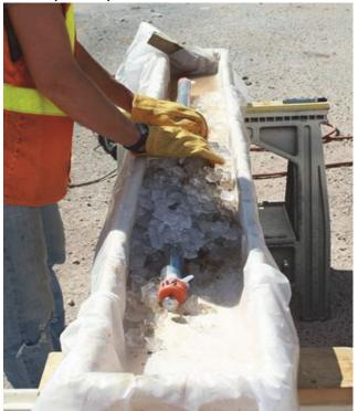
Hot sampling can also supplement temperature and power distribution data to allow discontinuation of heating of zones that have met cleanup goals, allowing power to be concentrated in zones not cleaning up as quickly.
