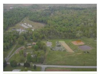
**Two Passive Treatment Systems:** Water is intercepted and diverted to the De Sale Phases 1 and 2 treatment systems where it is conveyed via gravity flow through multiple passive treatment steps.
