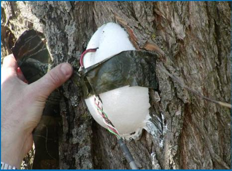
Based on correlation between sap flow and rate of heat dissipation in sapwood
