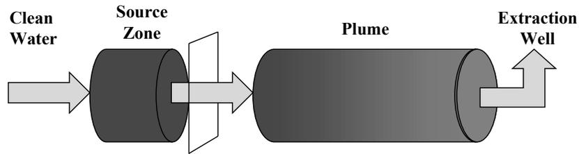
$$\text{Remediation Time} = \frac{\text{Source Zone Mass}}{\text{Exiting Flux} \cdot (A)}$$
