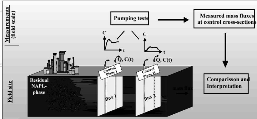
$$NA \text{ Rate} = -\ln \left( \frac{\text{Mass Flux (ControlPlane II)}}{\text{Mass Flux (ControlPlane I)}} \right) * \frac{1}{\Delta t}$$
