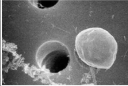
*Cryptosporidium* oocyst on upper surface of a 3  $\mu$ m pore
