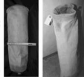
Figure 6-7 and 6-8. Bag filters showing discoloration associated with bypass.
