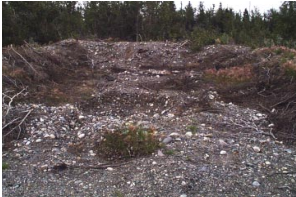
Figure 8. Revetment that concealed one of the tank targets used in SADARM tests. We collected one composite sample along the wall of the revetment and one from the floor of the revetment.
