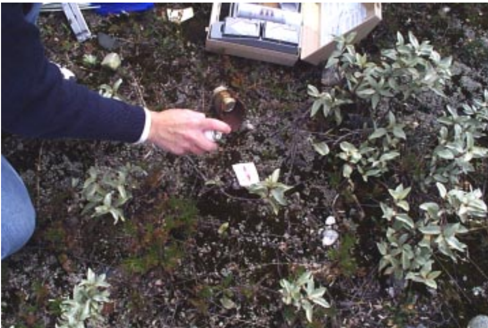
Figure 20. Using the Expray kit to identify the explosive filler of a 2.75-in. rocket warhead as Composition B.
