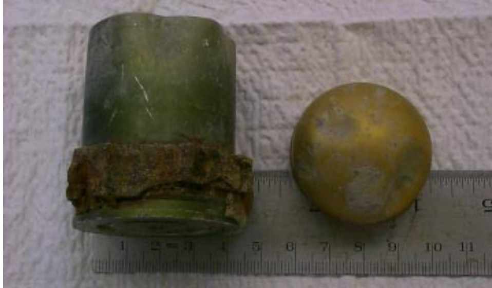
Figure 12. Cartridge case and ogive of a 40-mm grenade that contained residues of RDX, HMX, and NG.
