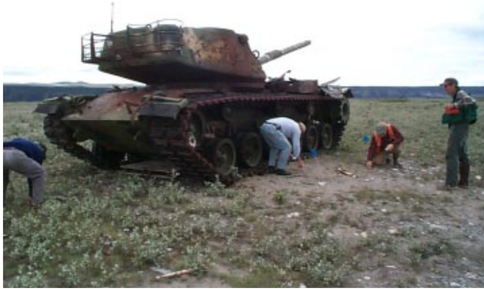
Figure 6. Tank used as a target during TOW missile tests. Six discrete samples were collected adjacent to the tank, then a series of composite samples were collected radially around the tank out to 50 m at 5-m intervals.
