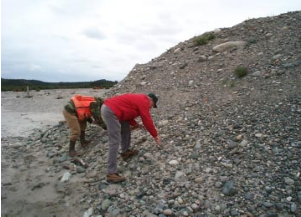
Figure 9. Impact berm for 40-mm grenade test. In November 1998, 1800 rounds were fired into this berm on the Lampkin Range.
