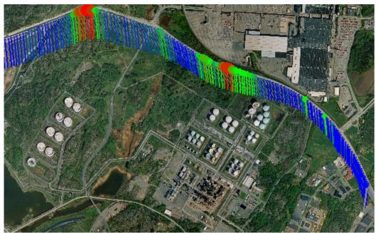
Figure 5. VOC measurements downwind a refinery. Red lines indicates points where high line integrated concentrations have been measured (maximum value 60 mg/m<sup>2</sup>) here). Blue lines indicate points with low concentrations. (Aerial photo: Copyright Lantmäteriet 2004-11-09. Ur Din Karta och SverigeBilden)
