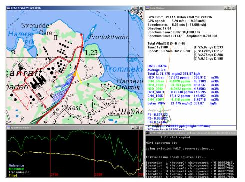
Figure 3. The screen of the measurement computer for the automatic retrieval software QESOF, developed for real-time evaluation of the measured spectra. In the upper left is shown a map of the measurement with lines pointing toward the wind, the measured and fitted absorption spectra in the lower left, and the retrieved data on the right side.
