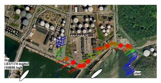
Figure 8. SOF measurements of two ships loading low volatile product class II, but with a previous high volatile cargo (class I). An emission rate of 125 kg/h was obtained. Red lines indicates points where high values have been measured here) while blue indicates low values. (*Aerial photo: Copyright Lantmäteriet 2004-11-09. Ur Din Karta och SverigeBilden*).
