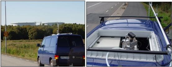
Figure 1. On the left the SOF car is shown while measuring emissions from crude oil tanks. The solar-tracker shown on the right transmits the solar light into the infrared spectrometer independently of the positioning of the car.
