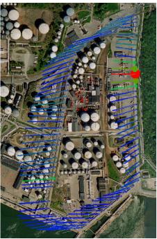
Figure 7. SOF measurements in an oilharbor is shown. Most of the leakages originate from a malfunctioning vapor recovery unit. Red lines indicates points where high values have been measured (maximum value 160 mg/m<sup>2</sup>) here) while blue indicates low values. (*Aerial photo: Copyright Lantmäteriet 2004-11-09. Ur Din Karta och SverigeBilden*).
