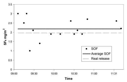
Figure 4. Results from a validation experiment in which  $SF_6$  was emitted from a 17 m mast at an open field and measurement with the SOF method were conducted. The average of the measured emissions was 11% higher than the real release rate.
