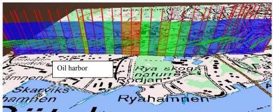
Figure 2. A 3D plot of a SOF measurement conducted at a oil harbor is shown. The red vertical lines correspond to solar lines. The colors in between the solar lines (blue to red) correspond to the integrated concentration of alkanes (blue is low concentration while green and red are higher). The wind vectors are shown as green horizontal lines pointing into the measurement-surface.
