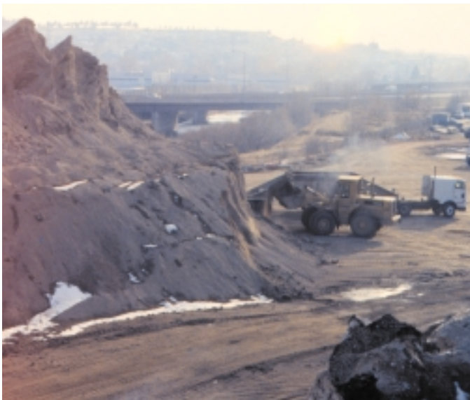
Figure 17. Recycled asphalt available for other projects (Recycled Materials Co.). Photograph by B. Arbogast.
