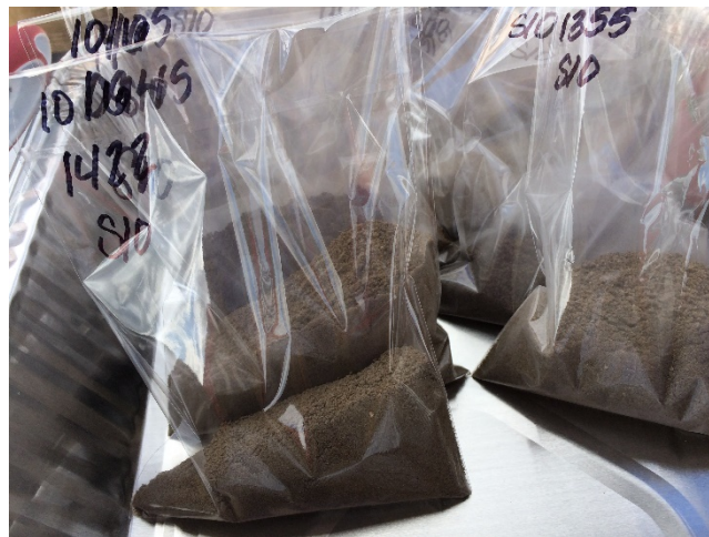
Sieved soil samples properly labeled and waiting XRF coarse readings.
