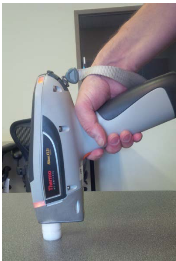
Figure 3: Reading standard without bag.
