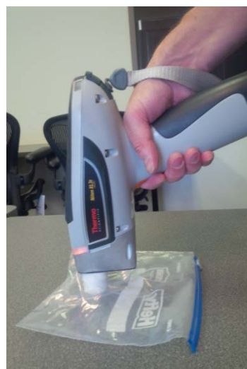
Figure 4: Reading standard with bag.
