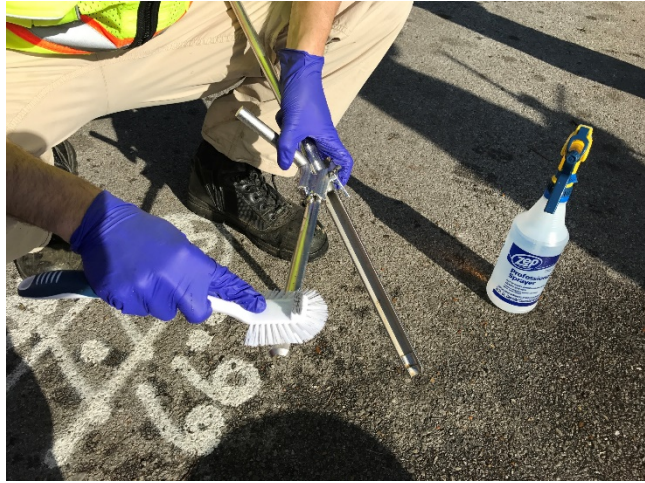
Decontamination of surface soil samplers.
