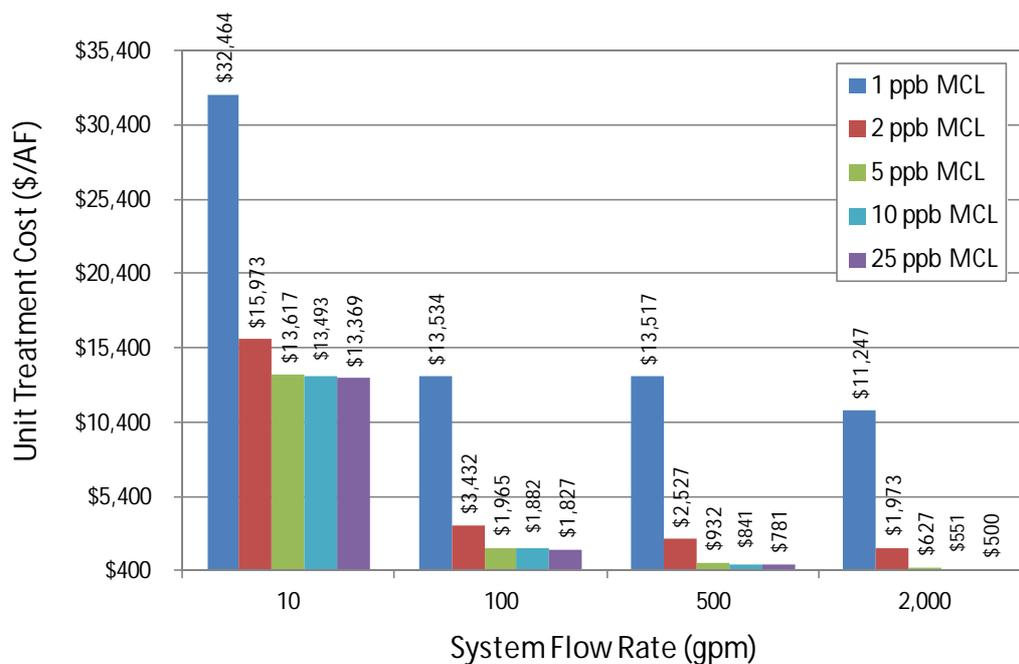
Figure 5-7. WBA Unit Treatment Costs Based on Total Cr Removal
