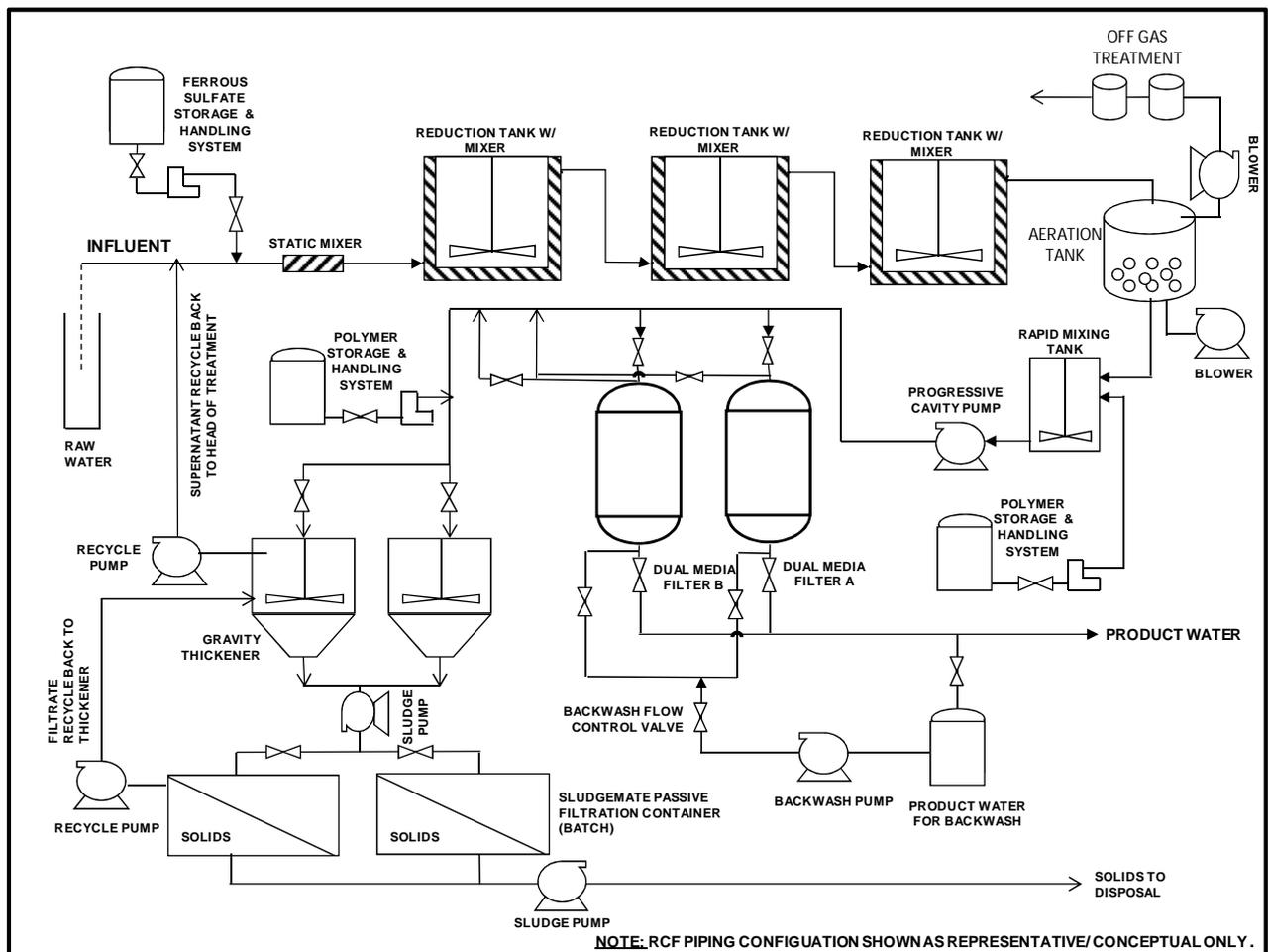
**Figure 5-8. Process Flow Diagram of 100-gpm RCF System**
