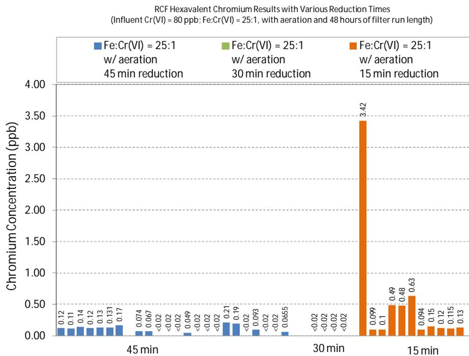
**Figure 4-14. Cr(VI) Concentrations in RCF Process Filter Effluent as a Function of Reduction Time**
