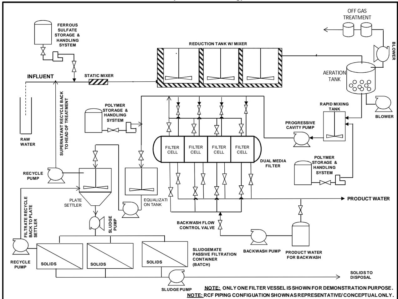
Figure 5-10. Process Flow Diagram of 2,000-gpm RCF System
