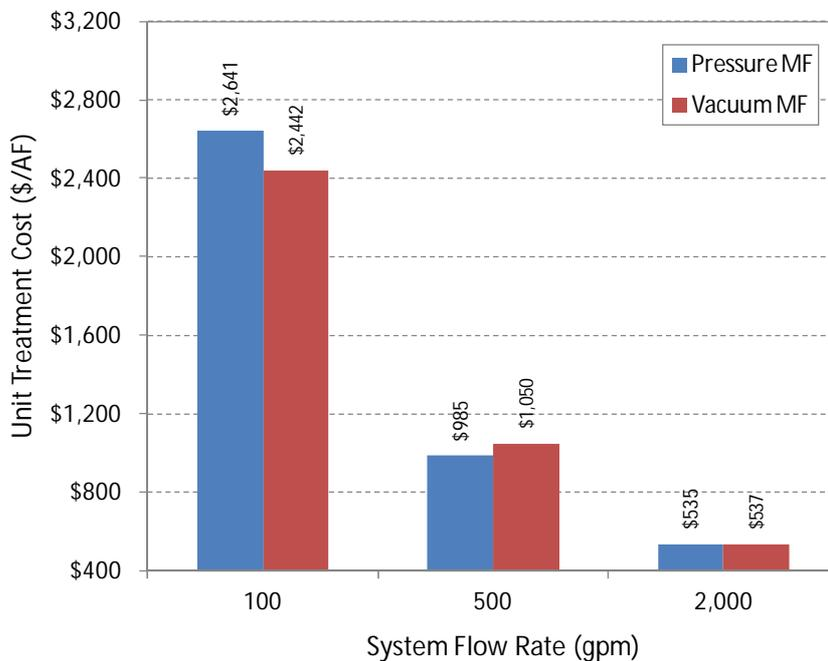
**Figure 5-17. RCF with MF Unit Treatment Cost**
