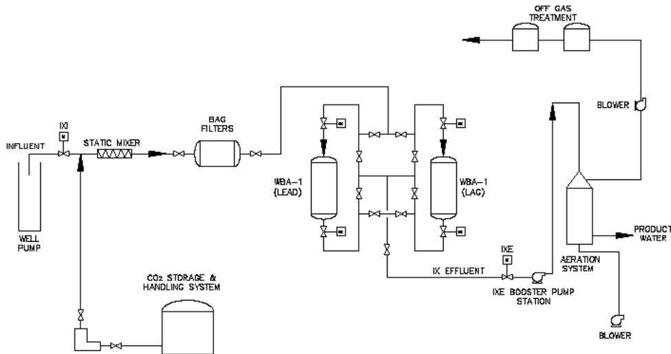
**Figure 5-2: Weak Base Anion Exchange Process Flow Diagram**
