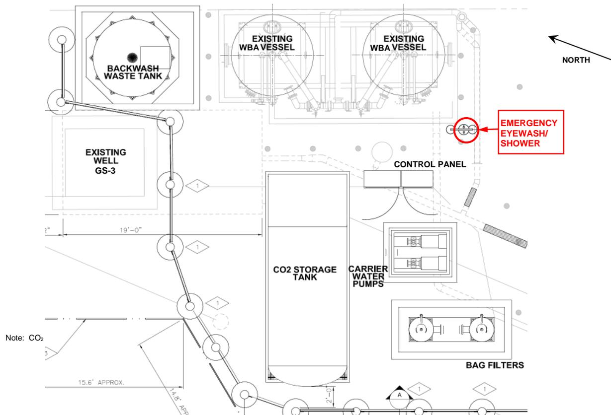
**Figure 4-2. Site Layout for the WBA Demonstration System**
