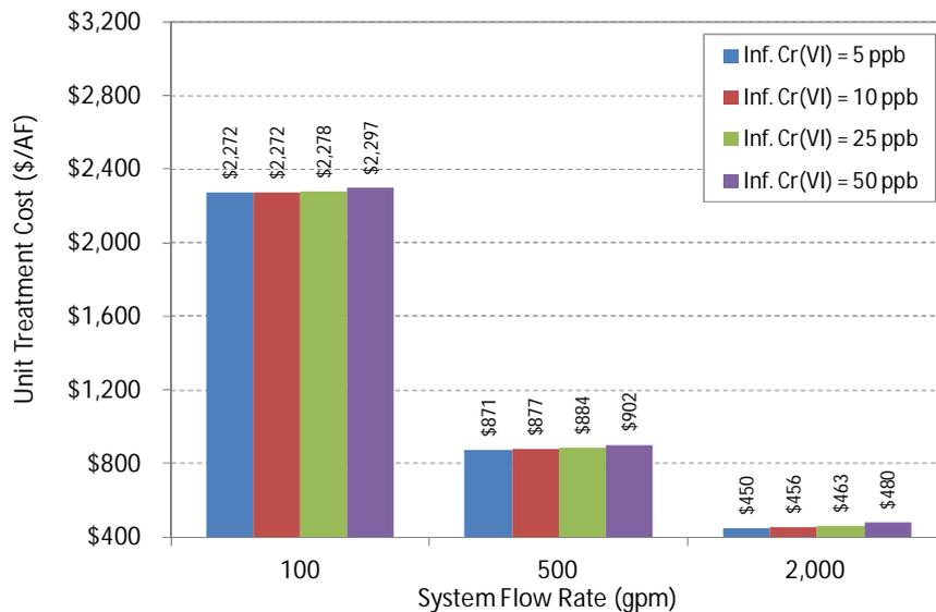
Figure 5-14. RCF without Recycle Unit Treatment Cost
