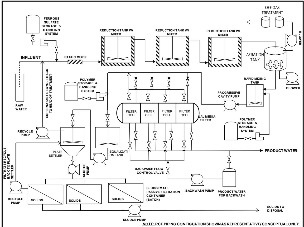
Figure 5-9. Process Flow Diagram of 500-gpm RCF System
