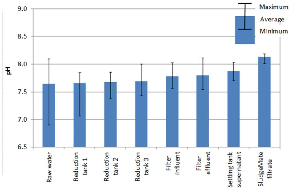
Figure 4-21. pH Values Through the RCF Demonstration Process
