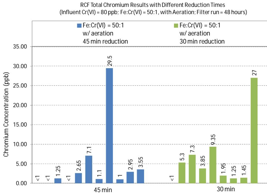
**Figure 4-17. Total Cr Concentrations in RCF Process Filter Effluent at a Higher Fe:Cr(VI) Ratio**
