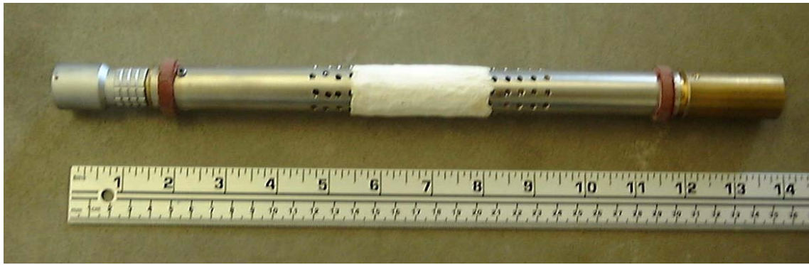
Figure 1. Photograph of the downhole XSD (halogen specific detector), which relies on oxidative chemistry. The sample vapors pass through a reactor core whose temperature is set in the range 800-1100 C, which is high enough to break C-Cl bonds. A current is induced as the chlorine atoms pick up electrons at a ceramic element that is doped with an alkali metal.
