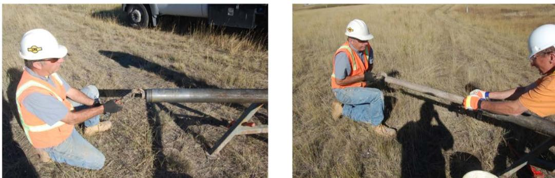
Figure 3-23. Extraction of Sample Liner
