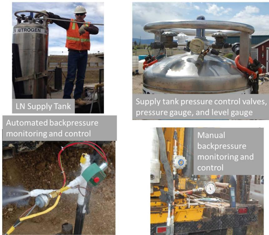
Figure 3-10. Liquid nitrogen set up
