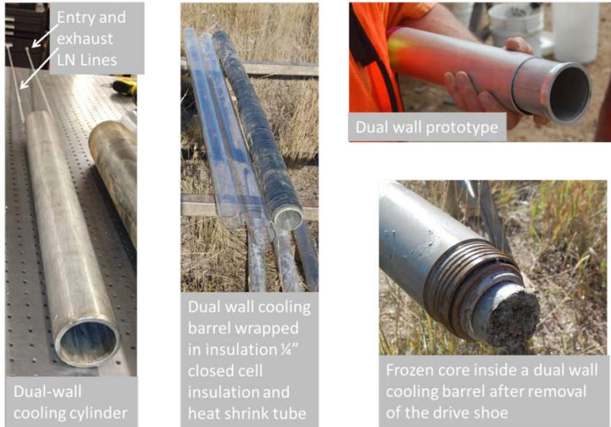
Figure 3-19. Dual-wall cooling cylinder
