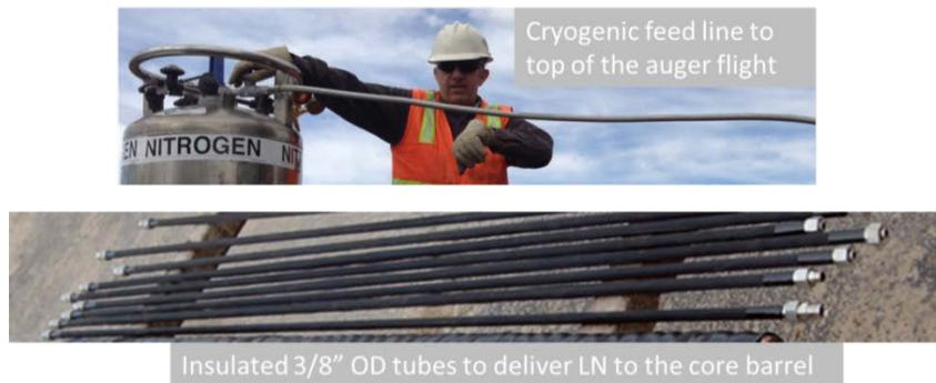
Figure 3-11. Liquid nitrogen supply and exhaust lines
