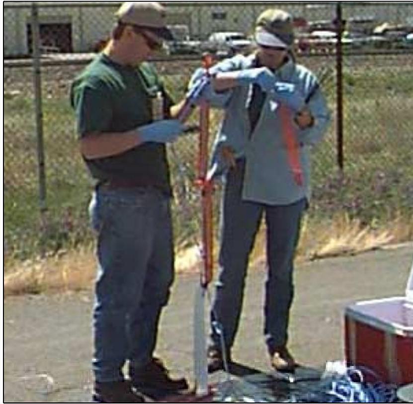
Figure 4.1. Installation of Diffusion Samplers into a Monitoring Well
