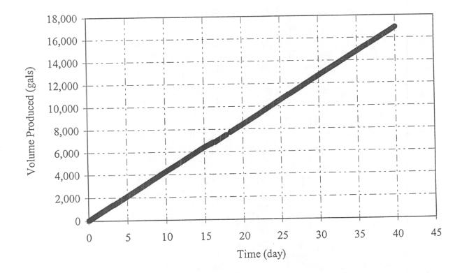
Figure M-24 Hydraulic control well HC02 cumulative volume injected as a function of time
