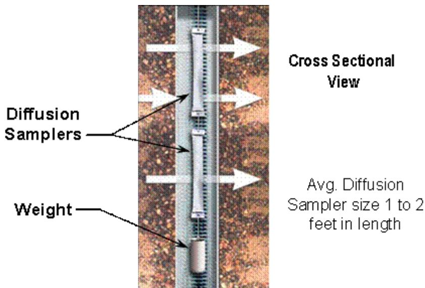
Recommendations for PDB sampler deployment vary with screen length:
