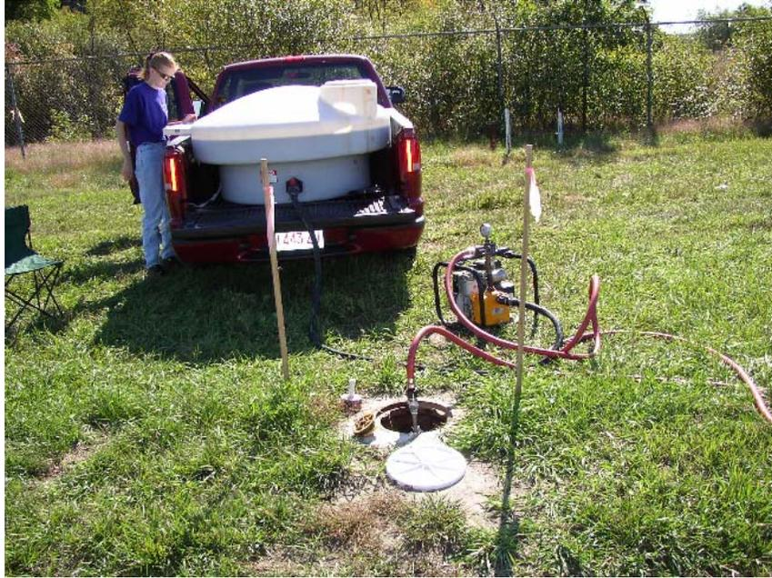
**Figure 4. Reagent Mixing and Injection System Photograph—HAFB.**
