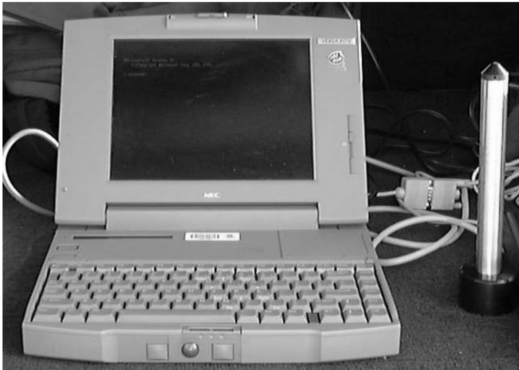
Figure 7.15 Photograph of downloading wireless pressure transducer data into a laptop computer using an optical reader.
