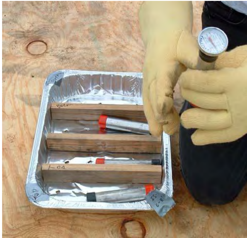
Figure 2. PVC Capped Sample Sleeves Ready for the Ice Bath
