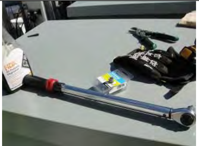
Figure 44 - Calibrated torque wrench
