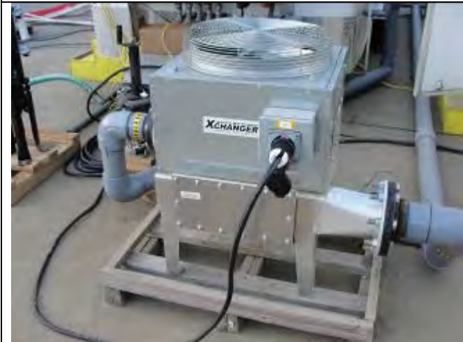
Figure 9 - Outside heat exchanger
