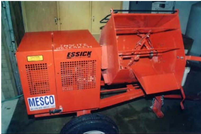
Fig. 3.7. Mortar mixer used for ATG demonstrations.
