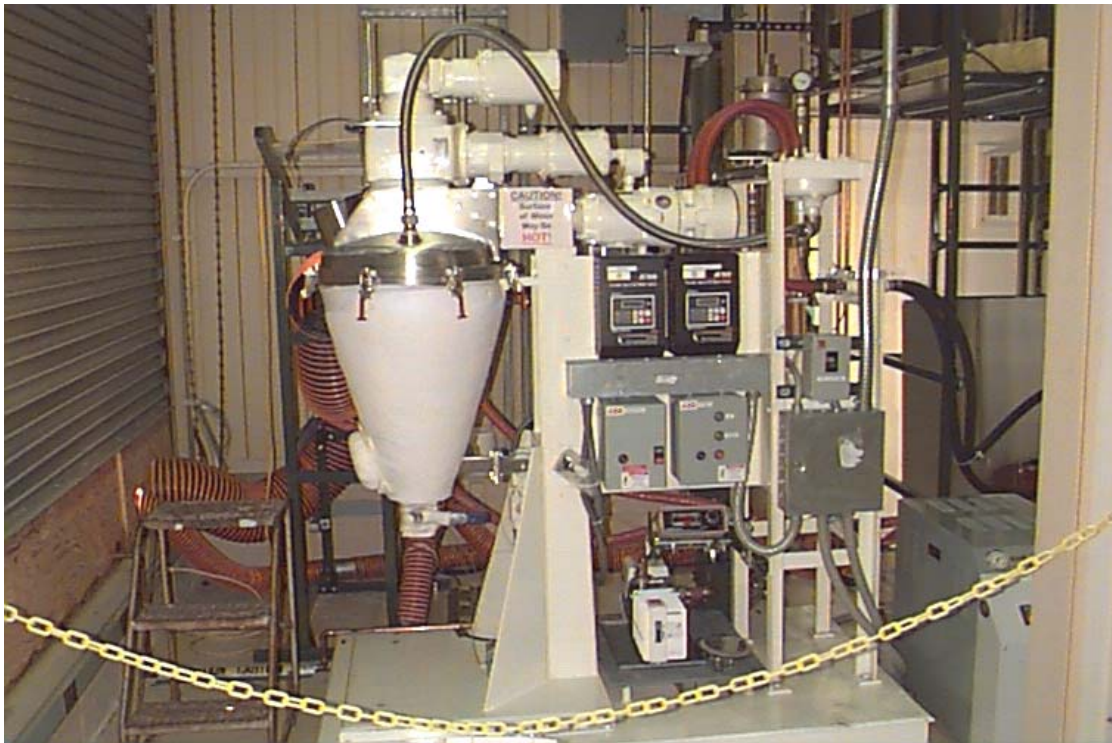
Fig. 3.1. SPSS mixer and process controls.
