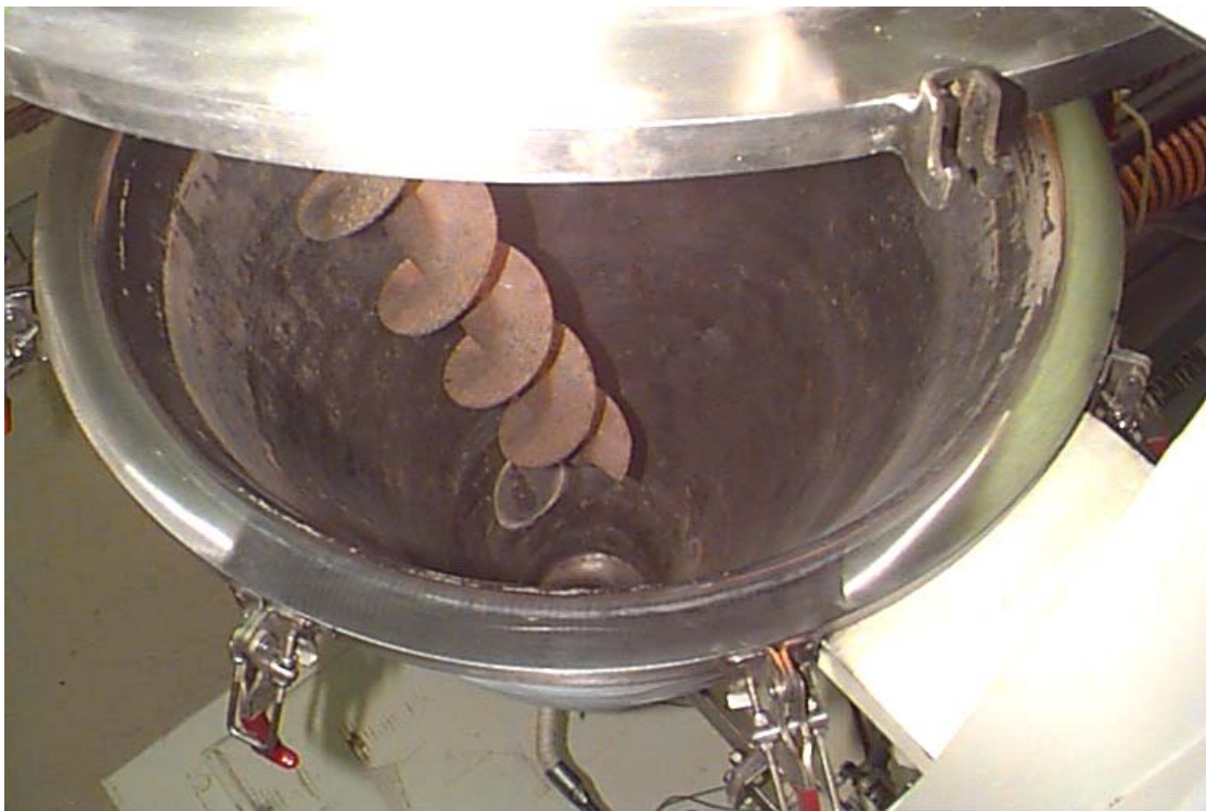
Fig. 3.2. View of inside of vertical cone mixer.
