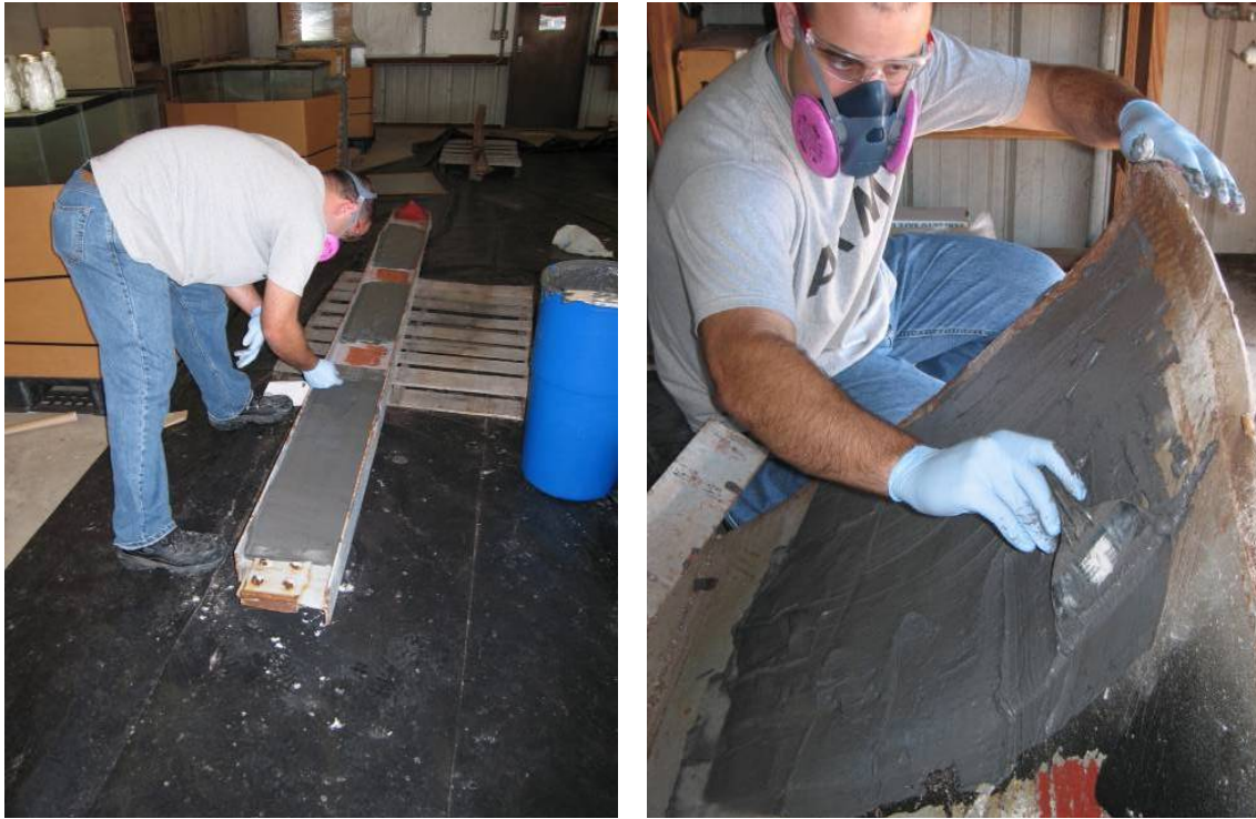
Figure 5-10. Manual application of BTS to VIB samples.
