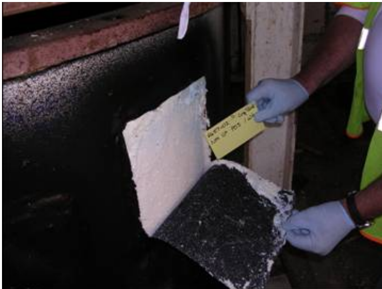
Figure 5-57. Sample being taken from large tank treated with NM-VP one week after application.
