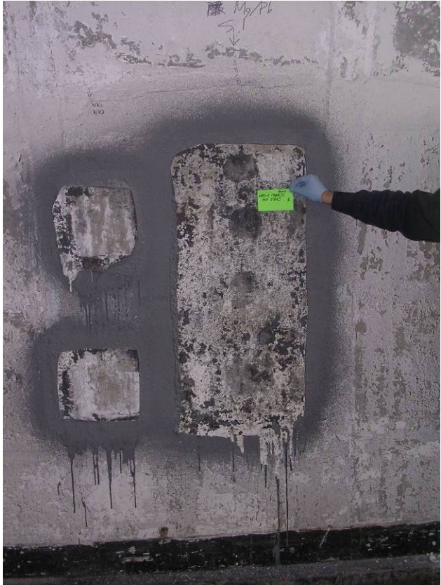
Figure 5-48. Mg/Pd-silicon after three week sampling event, 6810-11.
