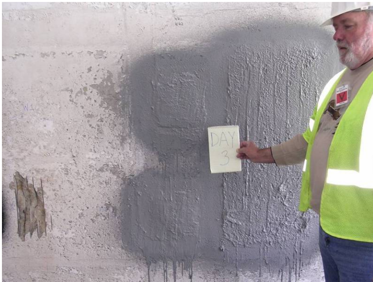
Figure 5-16. Three days post BTS application, Mg/Pd-silicon in 6810-11.
