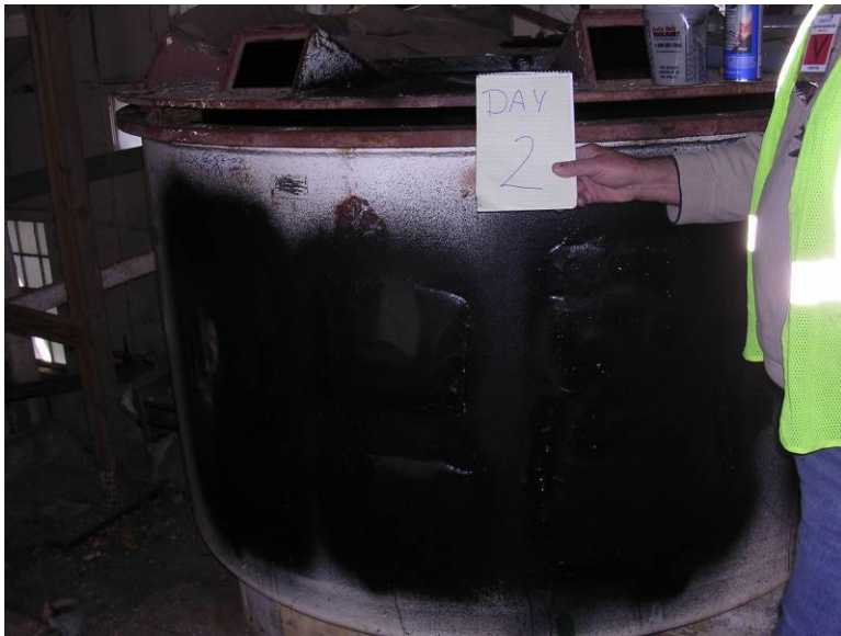
Figure 5-26. Large tank treated with Mg/Pd-VP and NM-VP, two days after application.
