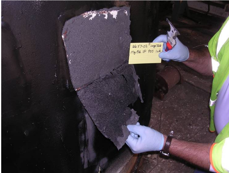
Figure 5-58. Sample being taken from large tank treated with Mg/Pd-VP one week after application.
