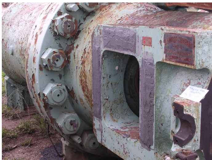
Figure 5-85. Quality of the paint on the presses in the staging area.
