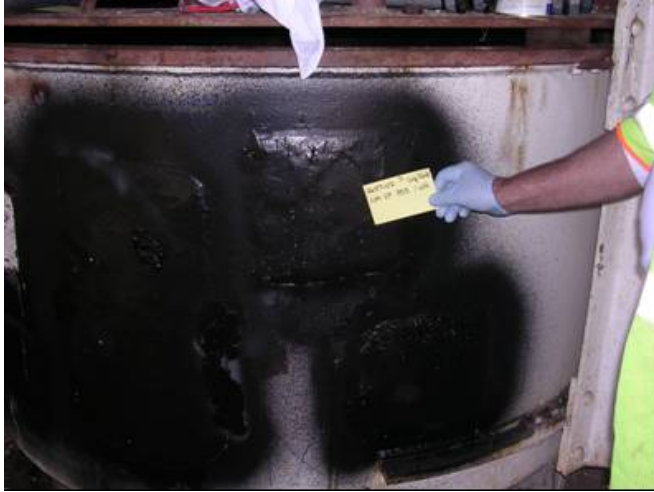
Figure 5-56. Large tank treated with Mg/Pd-VP and NM-VP one week after application.
