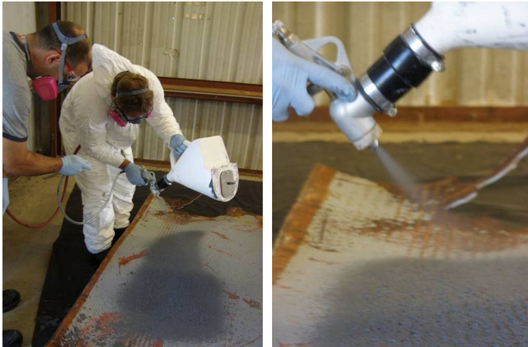
Figure 5-9. Application of BTS to VIB samples using pressurized sprayer
