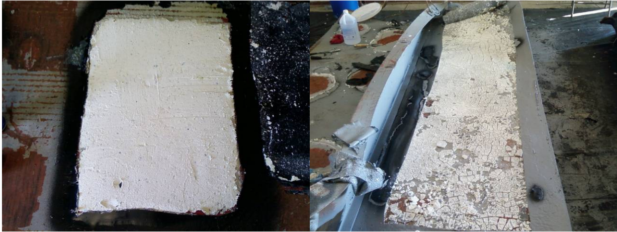
Figure 5-35. Varying appearance of BTS (non-metal paste) after exposure to paint and removal of sealant.
