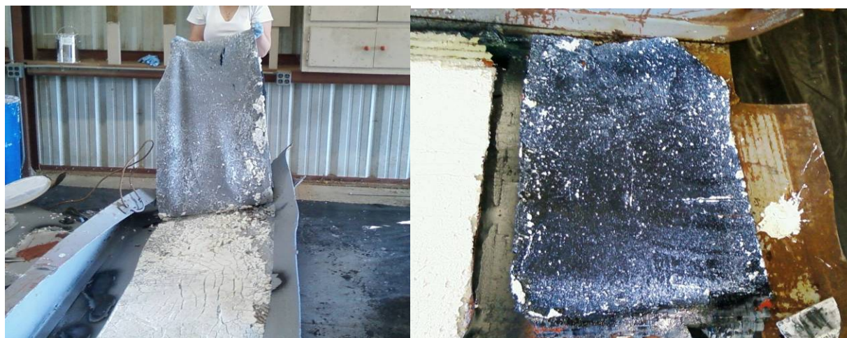
Figure 5-34. Removal of coating material after exposure to BTS
