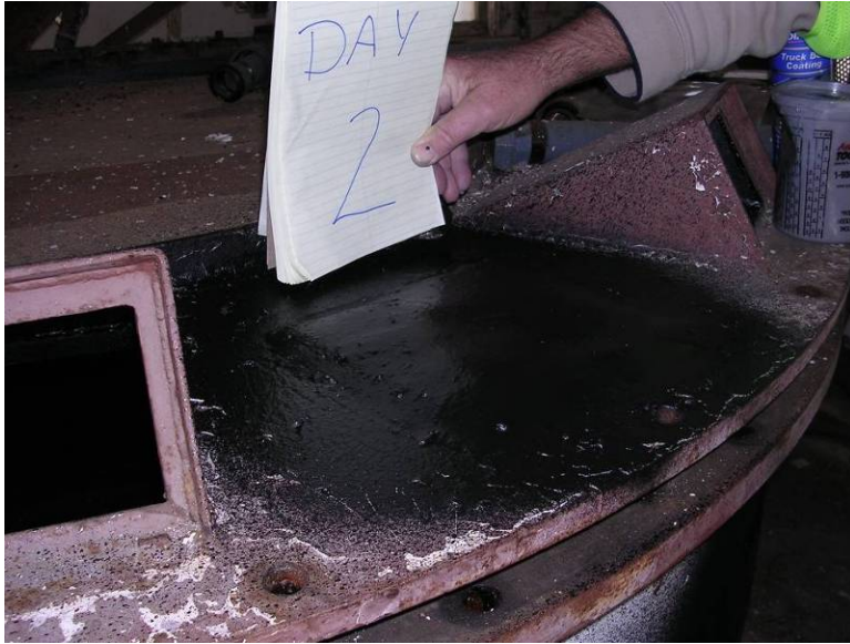
Figure 5-27. Large tank lid treated with Mg/Pd-VP, two days after application.
