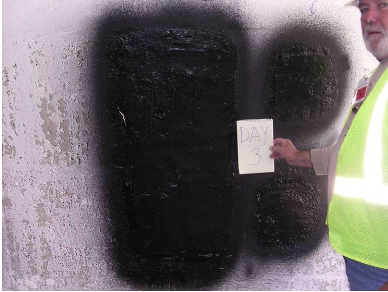
Figure 5-15. Three days post BTS application, NM-VP in 6810-11.
