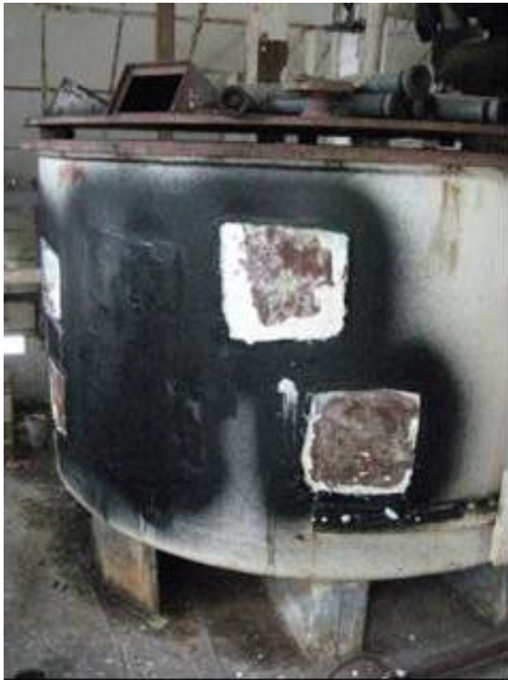
Figure 5-61. Large tank after sample was taken for two weeks of treatment.
