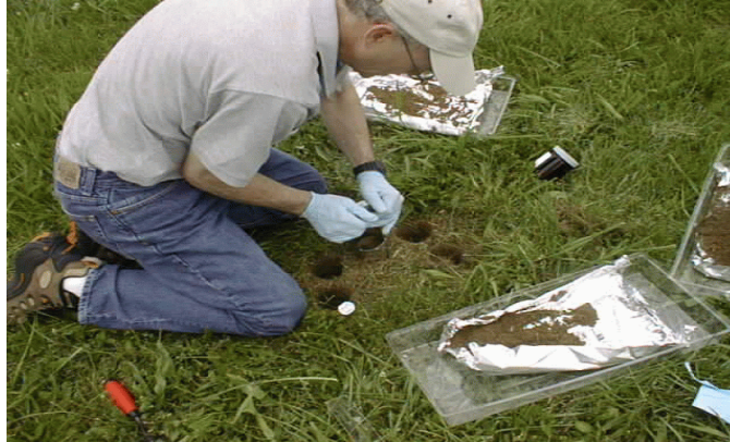
Picture 2. Sampling Using the Bulb Planter Method
